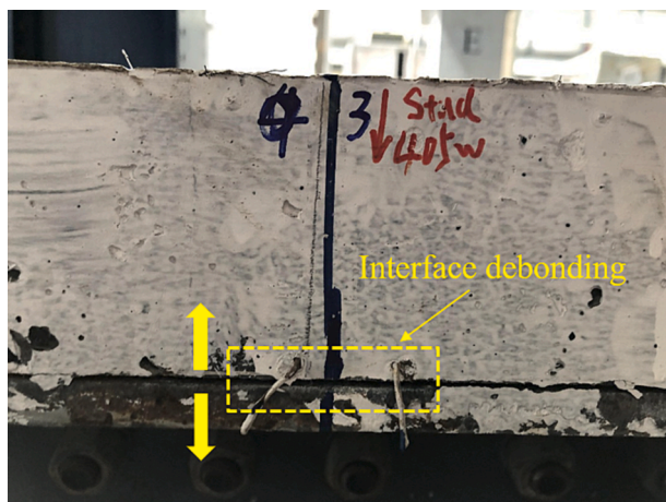
Fig. 16. Interface debonding at 3-N.
