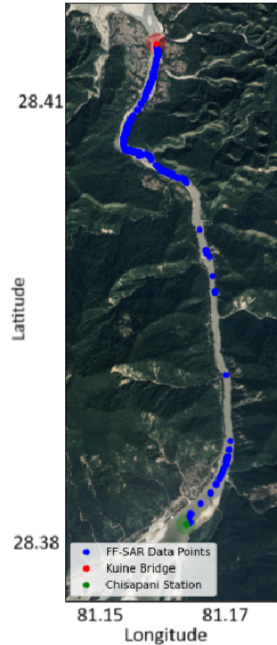
Figure 20: FF-SAR data points for a segment of the Karnali River in Bardiya National Park, Nepal. The locations of Kuine Bridge (red) and Chisapani river gauge station (green) are illustrated with circles representing the maximum allowable distance for the FF-SAR points.
