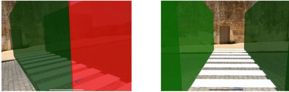
Figure 6: Concept 6. Left: non-yielding state with the closed red gate ‘blocking’ the pedestrian. Right: yielding state, where the gate is green and opened.
