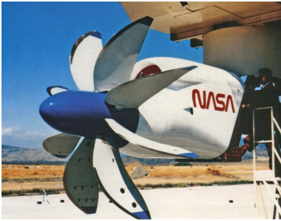
(a) PTA propfan concept developed by Lockheed for the NASA Advanced Turboprop Project [2].
