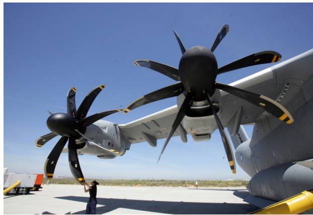
(c) TP400 turboprop developed by Europrop currently used on the Airbus A400M [4]
