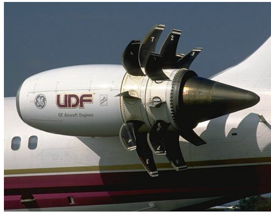
(b) Unducted Fan (UDF) developed by G.E. for the NASA Advanced Turboprop Project [2].
