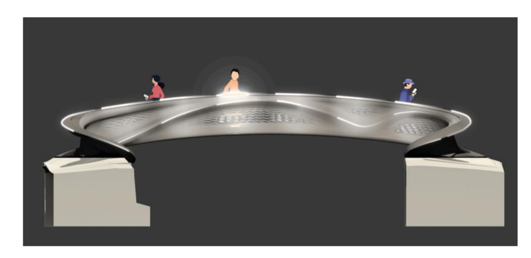
The resulting solution consists out of an animation controlled by data from the bridge that elicits the feeling of movement and annoys people away who are standing still. Hardware consisting out of projection mapping and custom designed LED handrail lighting enables the animation to be displayed on the sides of the bridge and the top of the handrail.
