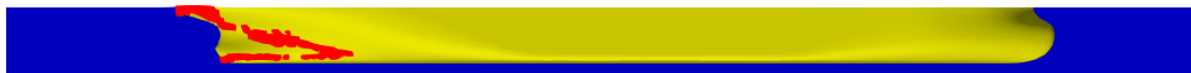
Figure 5.6: Residuals for \omega that are larger than 0.1 (red) are at the aft of the vessel.
