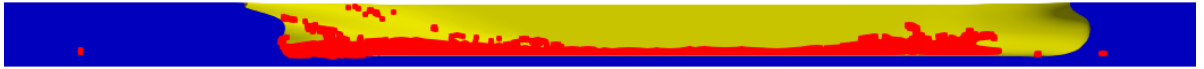
Figure 6.4: Residuals for water volume fraction c that are larger than 0.01 (red) with a thick Newtonian mud layer.
