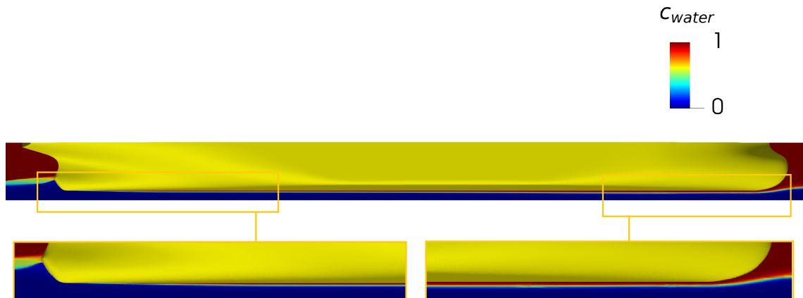
Figure 6.16: Water volume fraction at the symmetry plane for a flow with a Newtonian mud layer with a density of \alpha = 1.2 and a thickness of \frac{h_2}{T} = 0.3 .
