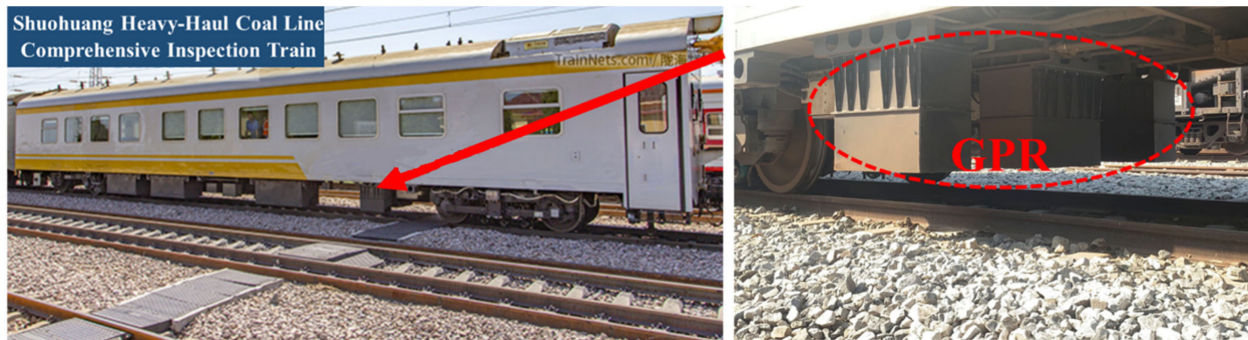
Figure 16. Integrated inspection vehicle with GPR system.
