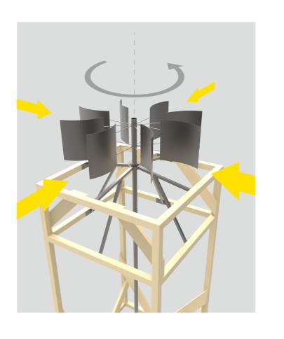
UpWind was designed based on a former design project. The sustainability impact of its life cycle was analyzed and improved. UpWind replaced the charcoal burner with a heat pump and replaced the plastic-coated drying racks with retired fishing nets. Moreover, UpWind utilizes natural resources, such as a wind-driven fan and chimney effect, to reduce the need for electricity.
