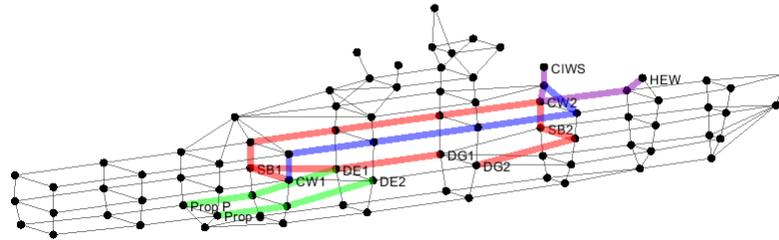
Figure 8: Physical location of the distributed systems networks in the adjusted conventional concept
