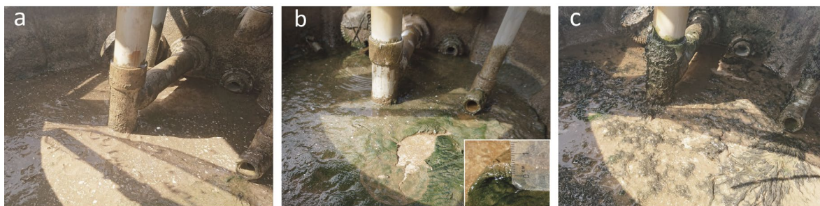
Figure 4.3. Deposits in the basin of the reference (a), P-limited (b) and non-P-limited (c) cooling towers at the end of the 5-week experiment.
