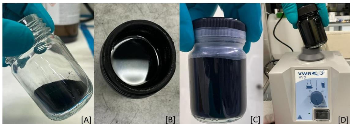
Figure 3.5: Fabrication process of the graphene nanoplatelets-based slurry. (A) Graphene nanoplatelets (B) Adding ethanol (C) Adding SPI carbon conductive paint and sealed with Parafilm (D) 10 minutes vortex mixing of the slurry.
