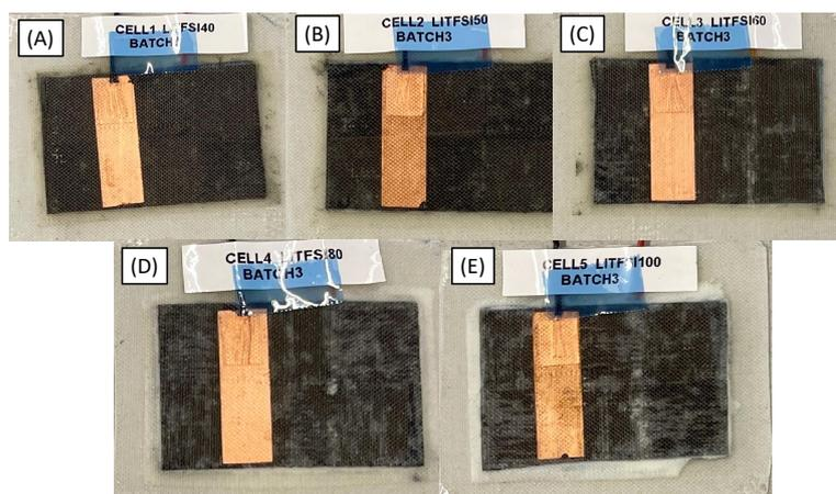
Figure 4.20: The image presents the change of the interface between the semi-cell and the glass fabric encapsulation when the LiTFSI concentration is increased in the gel polymer electrolyte. (A) to (E) are batch 3 cells 1 to 5. The whitened locations indicate the contact of the epoxy and the gel polymer electrolyte. As the LiTFSI concentration increases, the whitened area also increases, indicating that there is a reaction between the epoxy and the LiTFSI ions.
