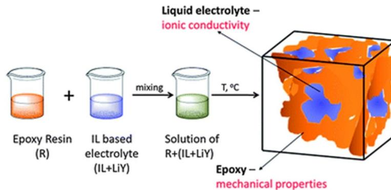
Figure 2.24: A schematic diagram of a reaction-induced phase separation method [118].
