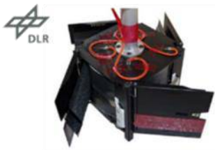
3U DLR-Surrey 'DeorbitSail' Deployer
