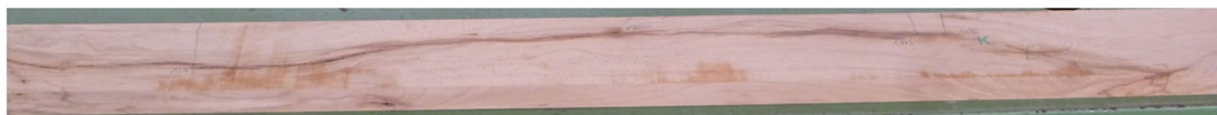
Fig. 8 Comparison of the tested and simulated parameters to the measured tensile strength and an example of beech board with extreme fiber deviation. (Left: simulated vs. actual dynamic MoE, right: predicted vs. actual tensile strength of the boards)
