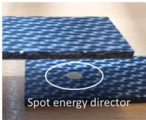
Fig. 5. Spot energy director fixed on composite adherend prior to welding process.
