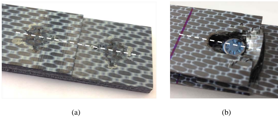
Fig. 17. Central-cut of both welded (a) and mechanically fastened (b) specimens along the dashed lines for the cross-sectional microscopy.
