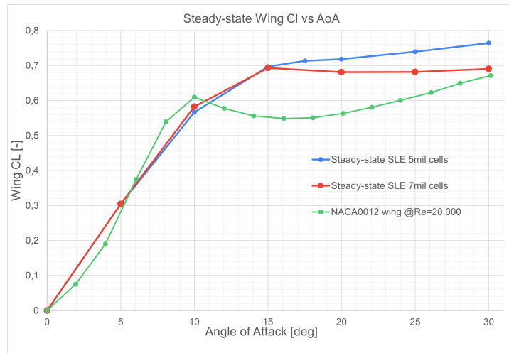
Figure 3.25: Effect of mesh refinement on steady-state lift curve
