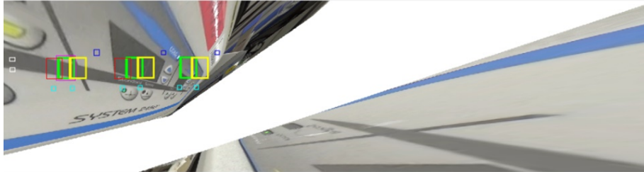
Fig. 13: Example of the incorrect perspective transformation after exceeding the limit of 35^\circ for the camera angle with respect to the normal of the screen.
