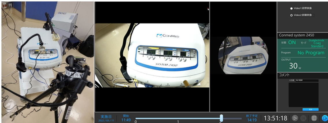
Fig. 22: Image of the setup for the fourth experiment. The image recognition system consisting of two cameras estimates the state of the Conmed System 2450. An additional camera and an endoscope provide extra visual data on the display of the Conmed. All results are shown on the decision-making navigation screen.
