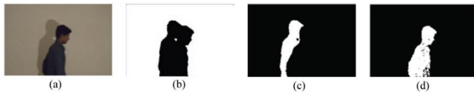
FIGURE 8: Detection process of an shadow withing an image with (a) the input image, (b) the subtracted background, (c) the detected shadow, and (d) the detected foreground. [102]
