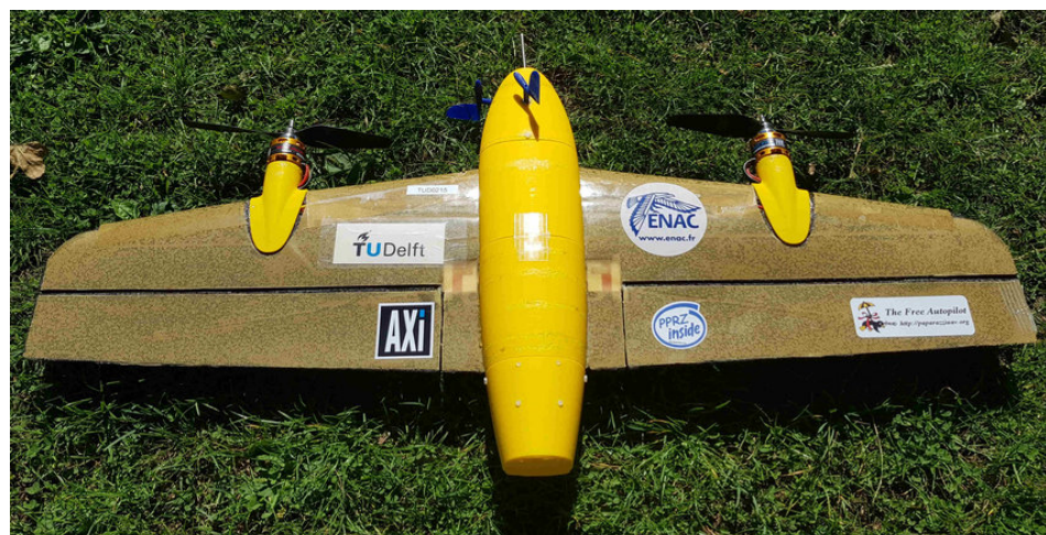
Figure 1. The Cyclone hybrid tail-sitter [19].
