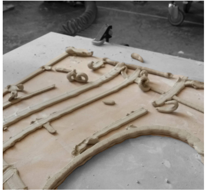
Fig.78. Left, the Dry consistency of the material caused discontinuous lines in relation to the robot speed. Right: curly lines resulted from the lack of viscosity and the water content in the mixture. (Source: Author)
