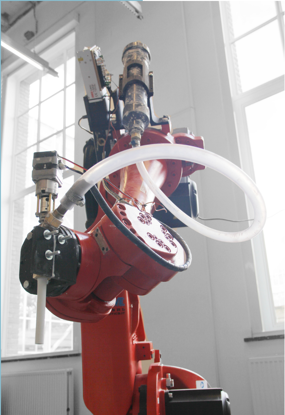
Fig.69. Fully assembled and mounted tools over the robot arm used for the printign process.(Source: Author)
