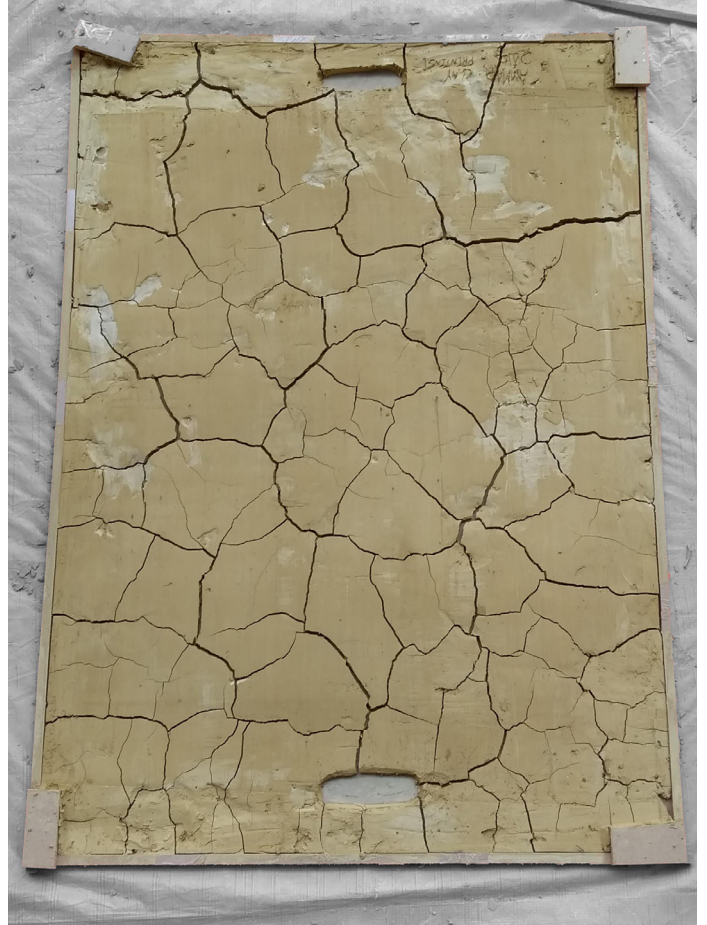
Fig.65. Left: Printing bed out of MDF Raised on a wooden platform, Right: Clay Plate casted as a trial for printing bed (Source: Author)
