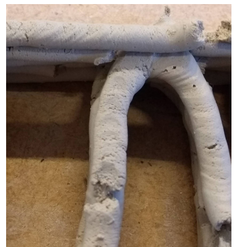
(c) Overlapping the infill on the long edges assures more stability
