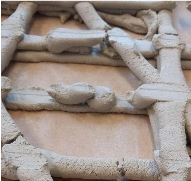
Fig.78. Left, the Dry consistency of the material caused discontinuous lines in relation to the robot speed. Right: curly lines resulted from the lack of viscosity and the water content in the mixture. (Source: Author)
