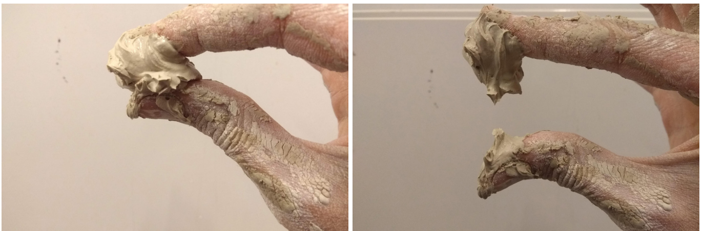
Fig.9. Plastic yet viscous material is better than the dry plastic one, this allows it to be sticky on the printing bed as well. iimage shows the inital extrudable consistency. (Source:Author)
