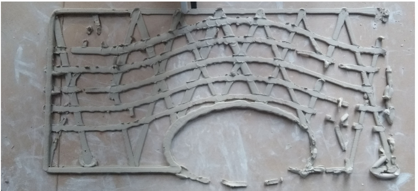
Fig.81. Discontinuous layer lines because of the clogging, the water percentage and the bed material. (Source: Author)
