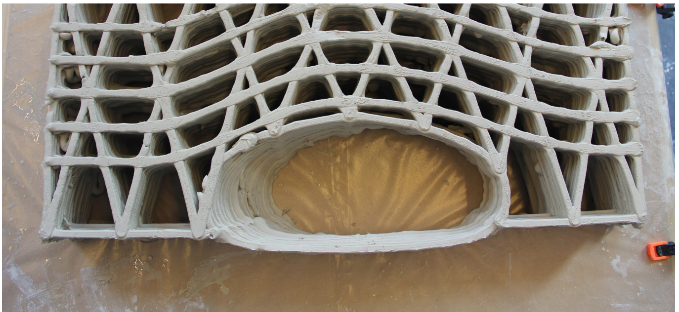
Fig.84. Top: Wooden MDF sheet caused crack, rapid shrinkage, un-planar printing and weak adhesion for the first layer. Bottom: Plastic cover sheet over the wood prevented the shrinkage and cracks while providing good adhesion for the first layer. (Source: Author)
