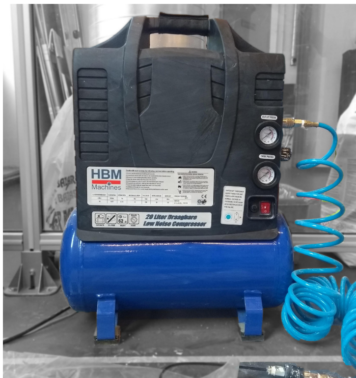
Fig.61. Top: PVC Pressurized cartridge used for feeding material through plastic hose, Bottom: Air compressor used to providing air to the cartridge. (Source: Author)
