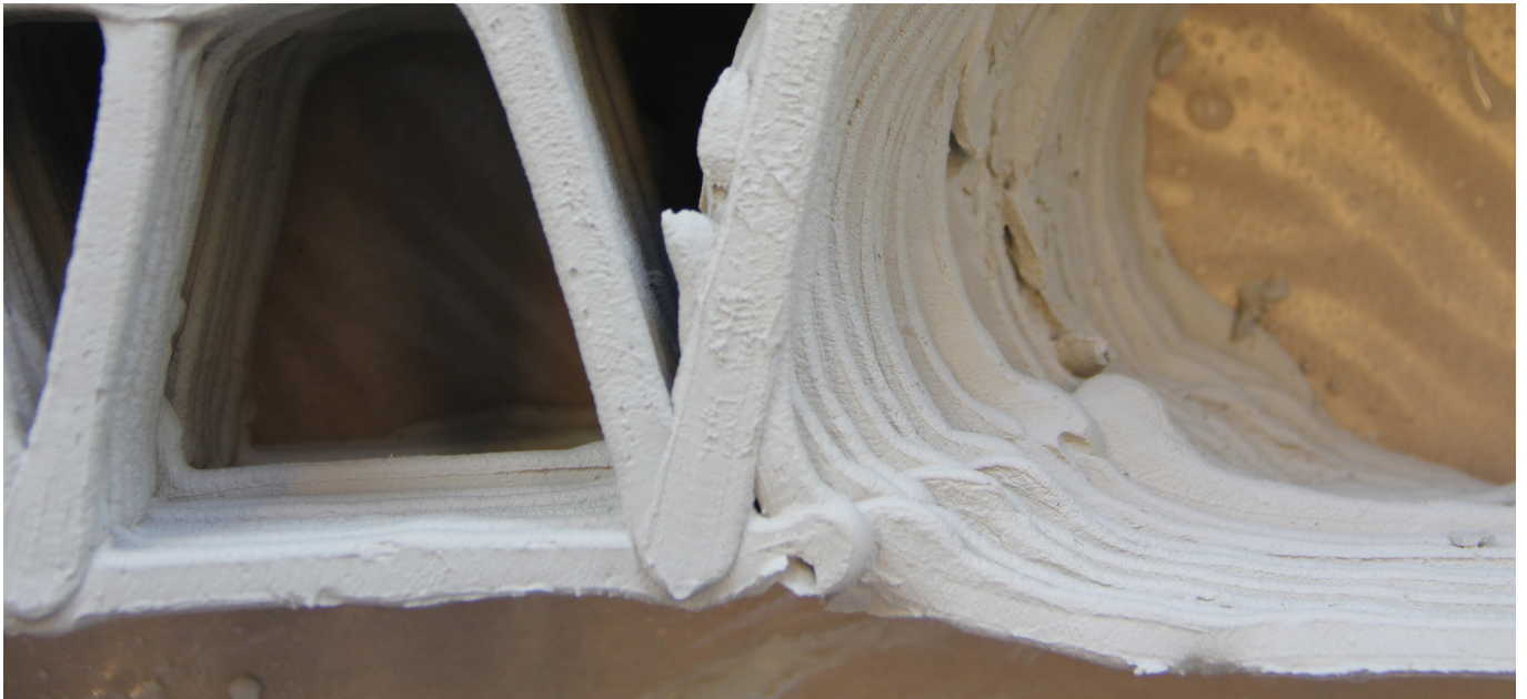
Fig.89. Top: The overhang of the duct has an angle which is enough to be supported without any structure supports. Bottom: Overlapping structure supports meets the duct at certain point and provide extra supports for it to be stable. (Source: Author)
