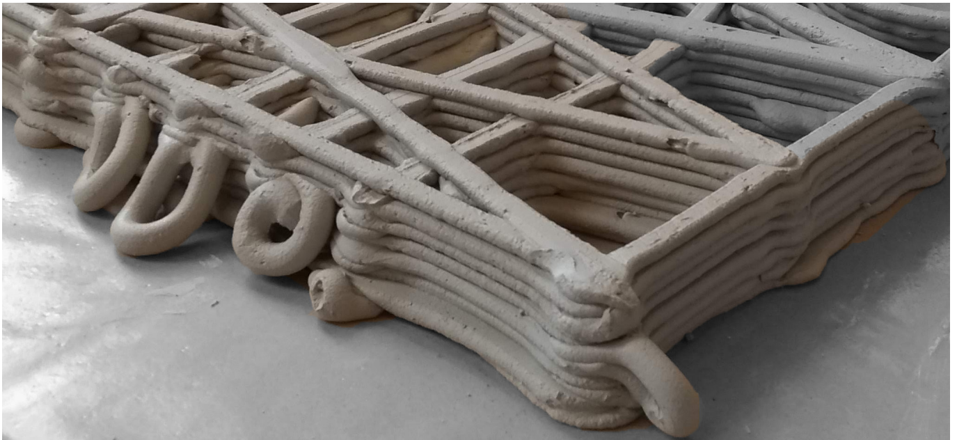
Fig.85. Excessive material on the outer surface and in the intersection nodes caused by the lack of I/O control to turn the motor on/off while printing. (Source: Author)
