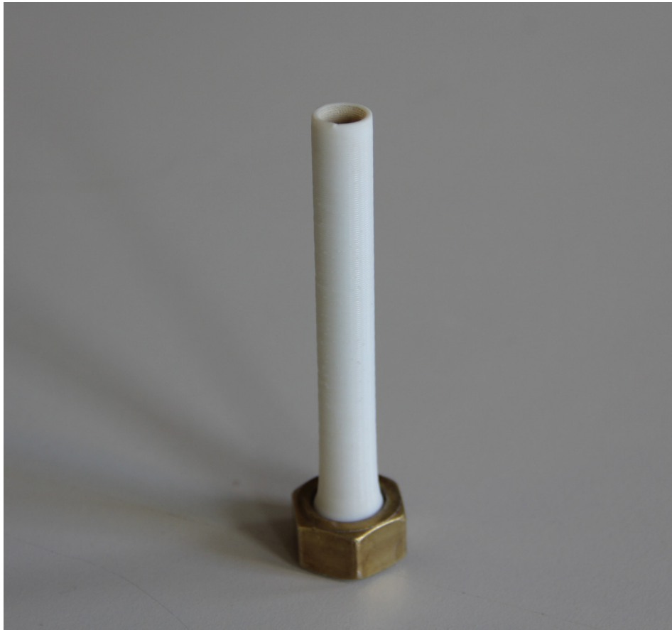
Fig.63. Top: digital model for the nozzle to fit within the metal thread, Bottom: PETG 3d printed nozzle used for extrusion , (Source: Author)
