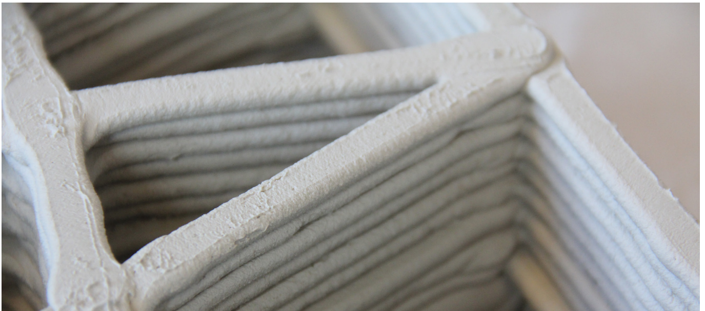
Fig.87. Top: Intersection nodes are recommended to be reduced to avoid material accumulation and cracks. Bottom: Overlapping the infilling with the layer boundary accumulates material as well and affects the outer surface quality. (Source: Author)
