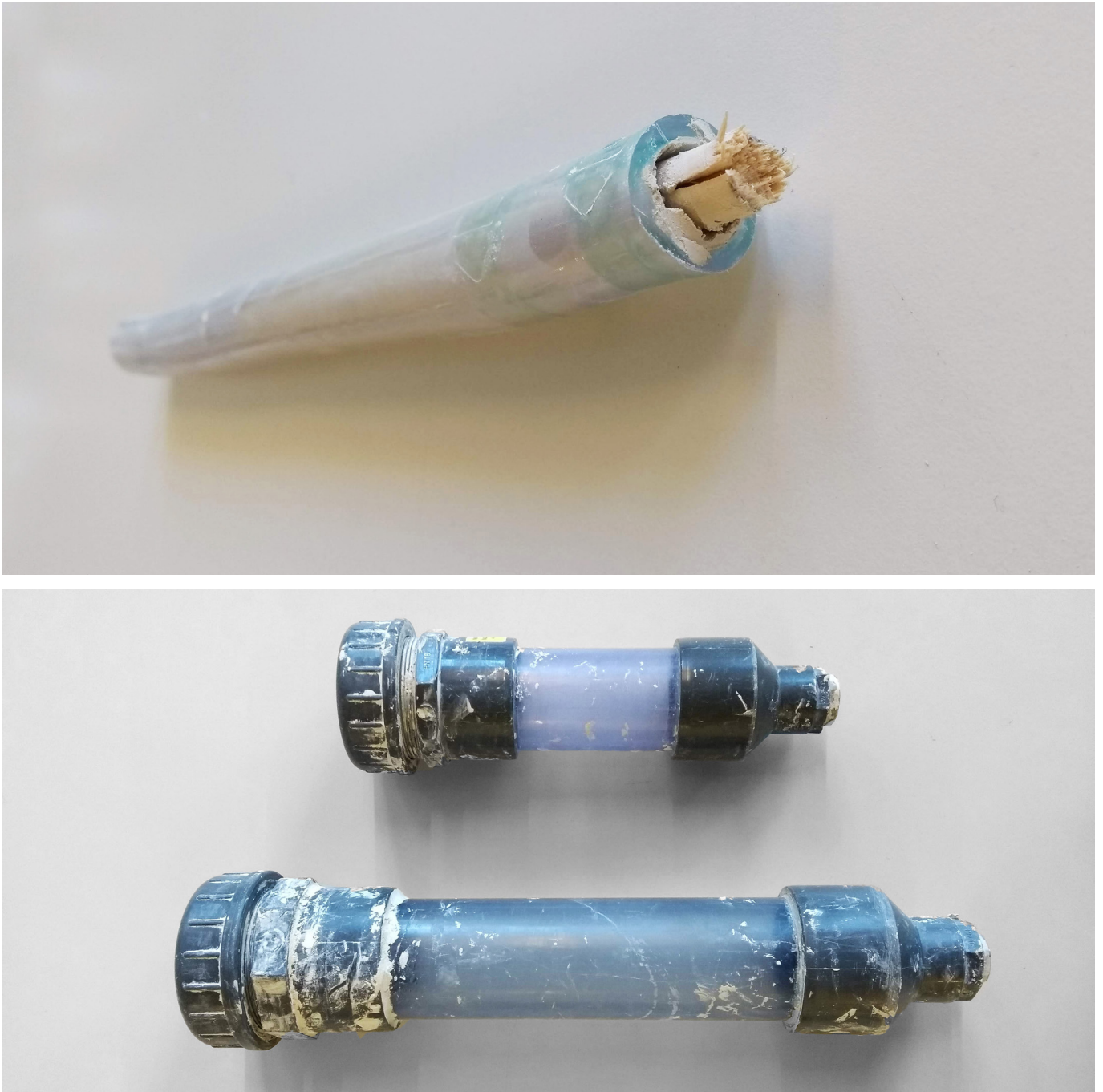
Fig.86. Top: the hose when gets stuck with dry material is almost useless and had to be cut shorter. Bottom: The two cartridge sizes used in the material feeding which were enough only for three layers in total to print. (Source: Author)
