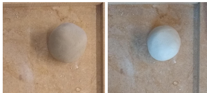
Fig.7. Clay balls were formed to weight before and after drying to estimate the weight loss (Source:Author)
