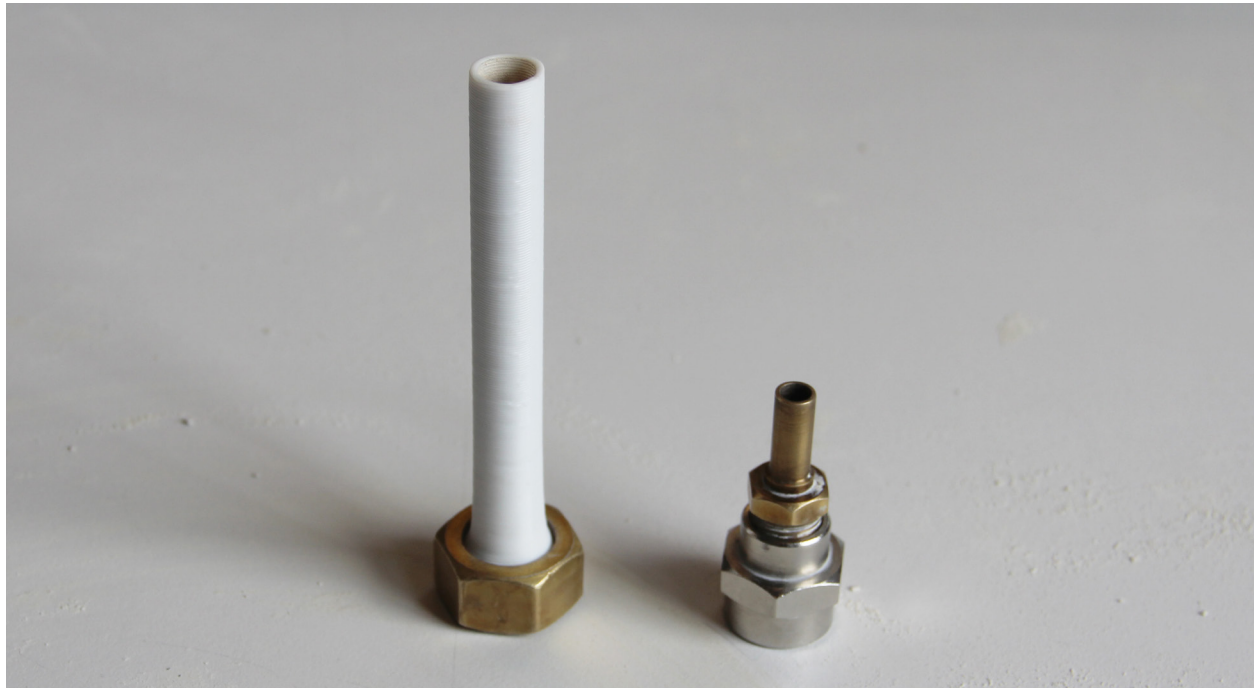
Fig.73. Used Nozzle size in material experiments had different requirements for the air pressure and the motor speed than the used nozzle size in the prototyping. (Source: Author)
