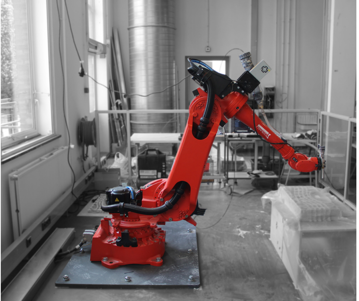
Fig.66. Used 6 axis Robotic arm Comau NJ6022 with a maximum reach of 2.2m. (Source: Author)
