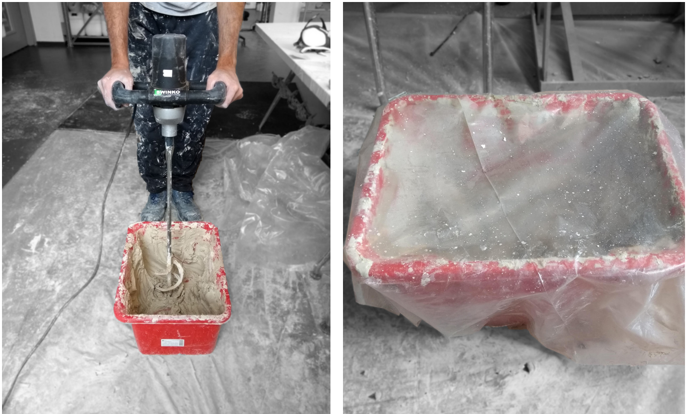
Fig.60. Left: Electric concrete mixer used for material preparation for printing, Right: covering mixture with plastic sheet keeps the mixture moist enough for printing over the week. (Source: Author)
