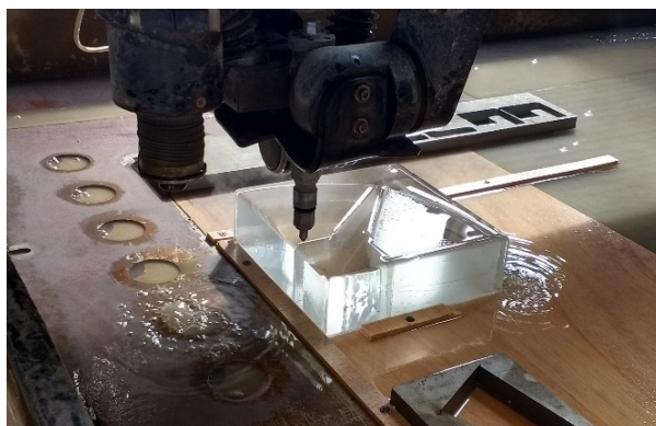
Figure 20: Waterjet cutting of the glass blocks for the nodes
