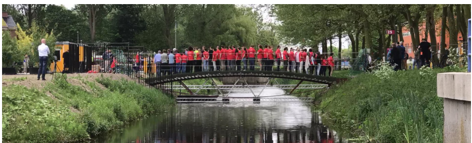
Figure 28 : Load case 1, 67 students, approximately 1.81 kN/m
