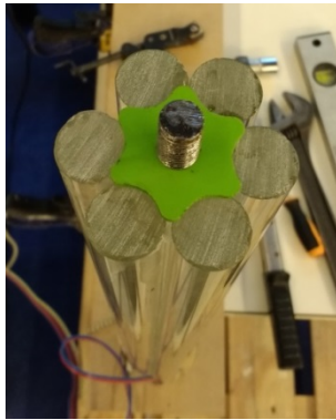
Figure 6: steel pre-tension rod and PLA centering ring
