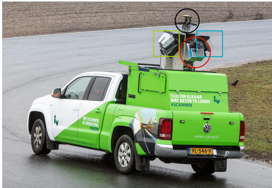
Figure 1.1: The mobile laser scan car of Iv-Infra include 3 laser scanners, 10 cameras for 360° photos, a GPS and an IMU system. The Z+F PROFILER 9012A is indicated with the red circle, the green and blue square indicates the Leica's P40 laser scanners. The black circle designates the GPS system and the 10 cameras for 360° photos.
