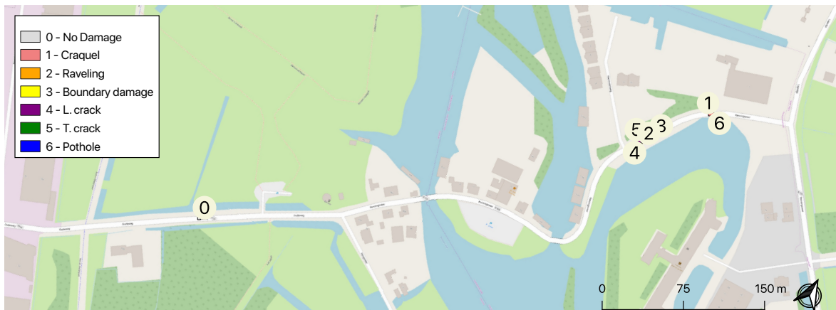
Figure 3.3: The research area with the locations of the damage of Figure 2.1. Number 0 represent an area with no damage, 1: craquel, 2: raveling, 3: boundary damage, 4: longitudinal crack, 5: transverse cracks and 6: potholes.
