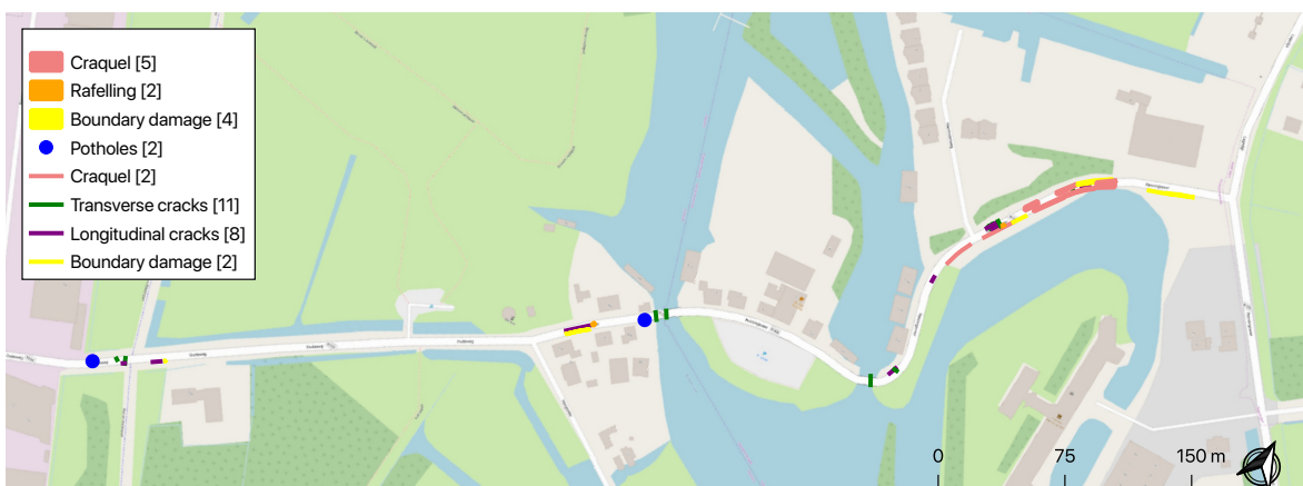
Figure 3.1: Research area, around 800 meters of the R106 near Haarlem, the Netherlands. On this road 36 damages were found by a road inspector. In this map, they are classified on damage type, and which shape (line, polygon or point) it was saved. Back ground map is from OpenStreetMap, (OpenStreetMap contributors, 2017)
