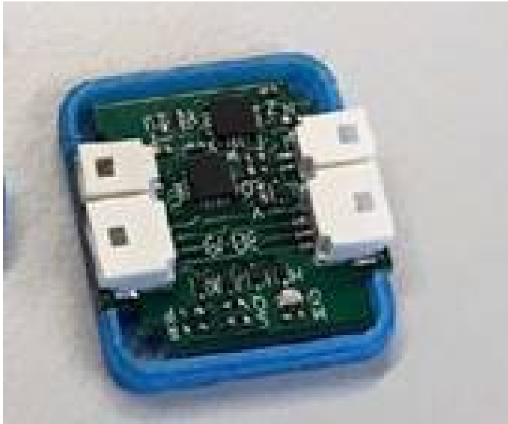
Figure 1.1: Sensor unit as used in 2020 version of the Sensor Shorts (21*24*8 mm) at the project CAS P6 of TU Delft
