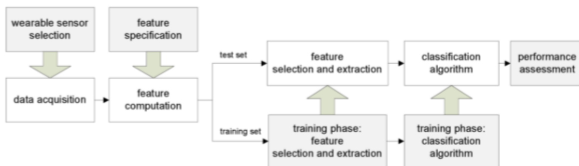
Figure 1.2: Schematic diagram for classification[13]
