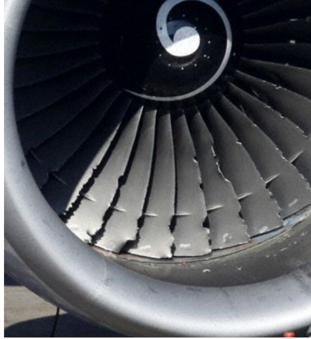
Figure 1-2 Engine inlet with fan damage
