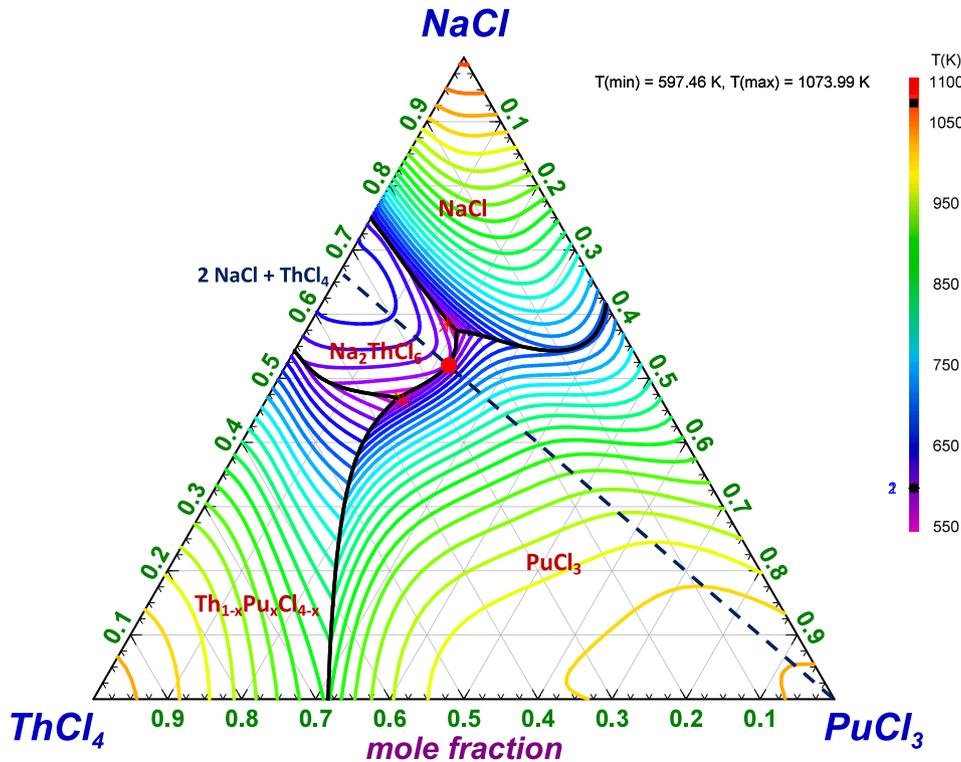
Fig. 5. Liquidus projection of the NaCl-ThCl<sub>4</sub>-PuCl<sub>3</sub> system assessed in this work from 550 K to 1100 K with an increment of 20 K. Primary crystallization fields are indicated in the figure: NaCl; Na<sub>2</sub>ThCl<sub>6</sub>; Th<sub>1-x</sub>Pu<sub>x</sub>Cl<sub>4-x</sub>; PuCl<sub>3</sub>. (\*) Positions of the ternary eutectics and (●) the eutectic on the (2 NaCl + ThCl<sub>4</sub>)-PuCl<sub>3</sub> pseudo-binary section measured by Desyatnik et al. [23].
