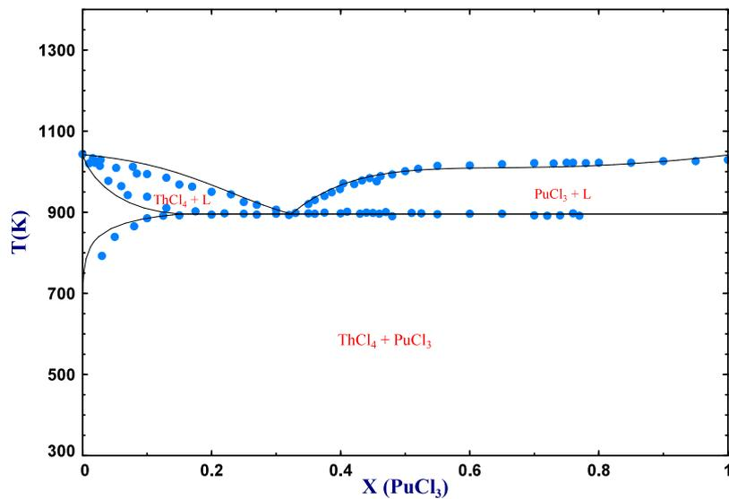
Fig. 3. Phase diagram of the ThCl<sub>4</sub>-PuCl<sub>3</sub> system modeled in this work. (●) Data from Vorobei et al. [8].
