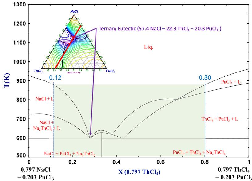
Fig. 9. Calculated pseudo-binary phase diagram of the 79.7 (NaCl-ThCl<sub>4</sub>) + 20.3 PuCl<sub>3</sub> system, intercepting the ternary eutectic determined in Section 3.4. The green area represents the range of compositions with a liquidus transition below the minimum safety temperature of operation (T = 873 K).
