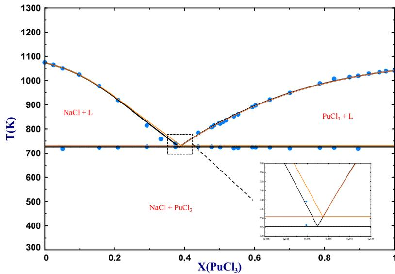
Fig. 1. NaCl-PuCl<sub>3</sub> phase diagram calculated in this work (—) and ● data from Bjorklund et al. [18]. The phase diagram (—) shown in orange is calculated from the previous model of Beneš and Konings [7].
