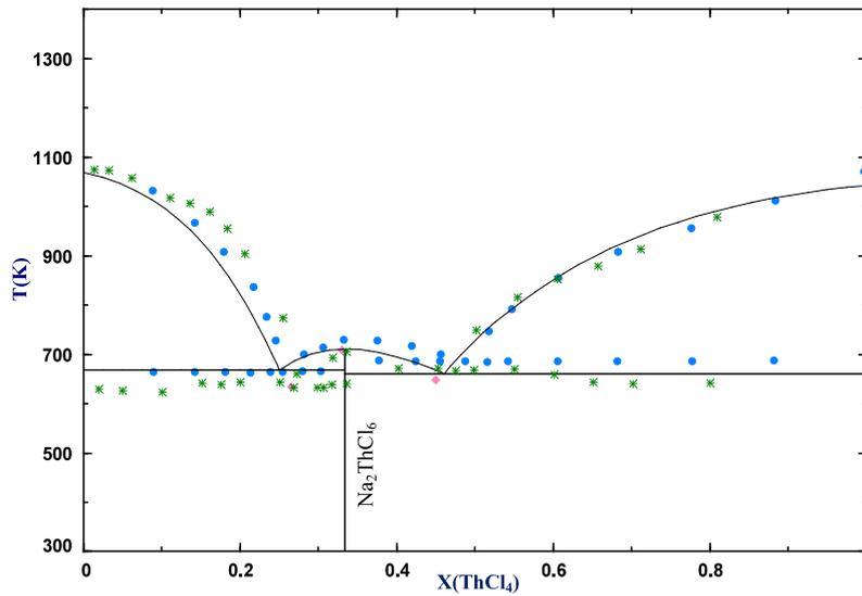
Fig. 4. NaCl-ThCl<sub>4</sub> calculated phase diagram by Ocádiz-Flores et al. [29], but excluding the low temperature metastable  $\alpha$  phase. (\*) Data from Tanii et al. [20], (●) data from Oyamada [21] and (◆) data from Vokhmyakov et al. [22].
