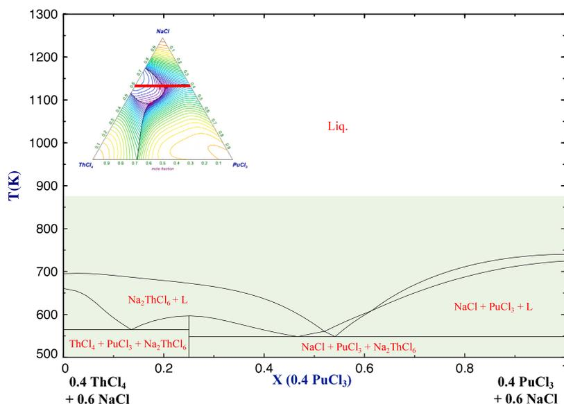
Fig. 11. Phase diagram of the pseudo-binary 40 ( $\text{ThCl}_4$ - $\text{PuCl}_3$ ) + 60 NaCl system with the composition area of safety with the minimum inlet temperature minus 50 K (873 K) superposed in green.
