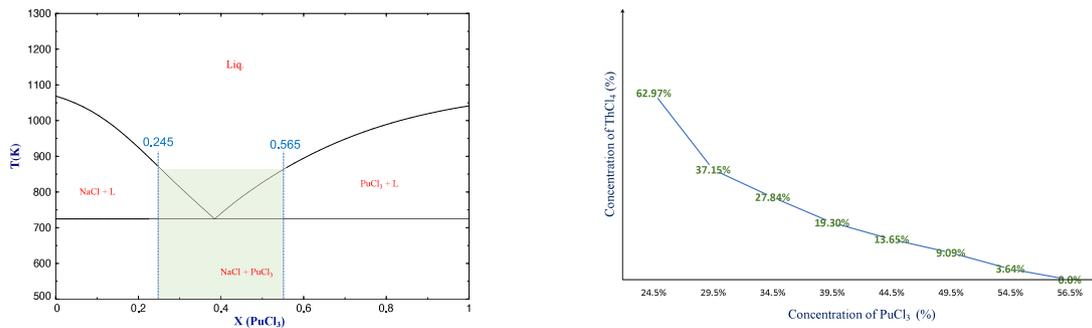
Fig. 7. Phase diagram of the  $\text{NaCl}$ - $\text{PuCl}_3$  system with the composition area of safety with the minimum inlet temperature minus 50 K (873 K) superposed in green (left), and curve of the maximal safe molar concentration\* of  $\text{ThCl}_4$  in the ternary solution  $\text{NaCl}$ - $\text{ThCl}_4$ - $\text{PuCl}_3$  as a function of the concentration of  $\text{PuCl}_3$ . \*Maximum concentration ensuring melting temperature of the ternary solution below 873 K.
