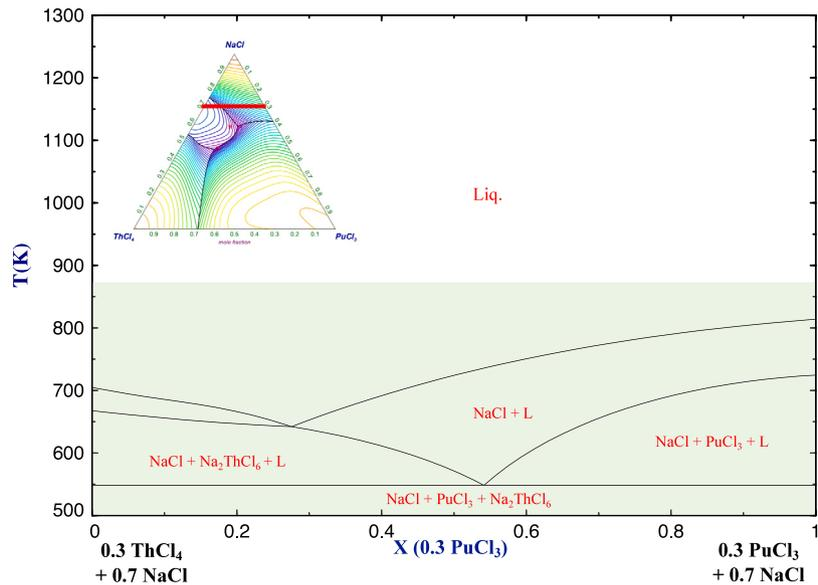
Fig. 10. Phase diagram of the pseudo-binary 30 (ThCl<sub>4</sub>-PuCl<sub>3</sub>) + 70 NaCl system with the composition area of safety with the minimum inlet temperature minus 50 K (873 K) superposed in green.
