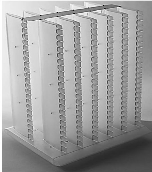
Figure 2 - Aerodynamic rake for seeding distribution.
