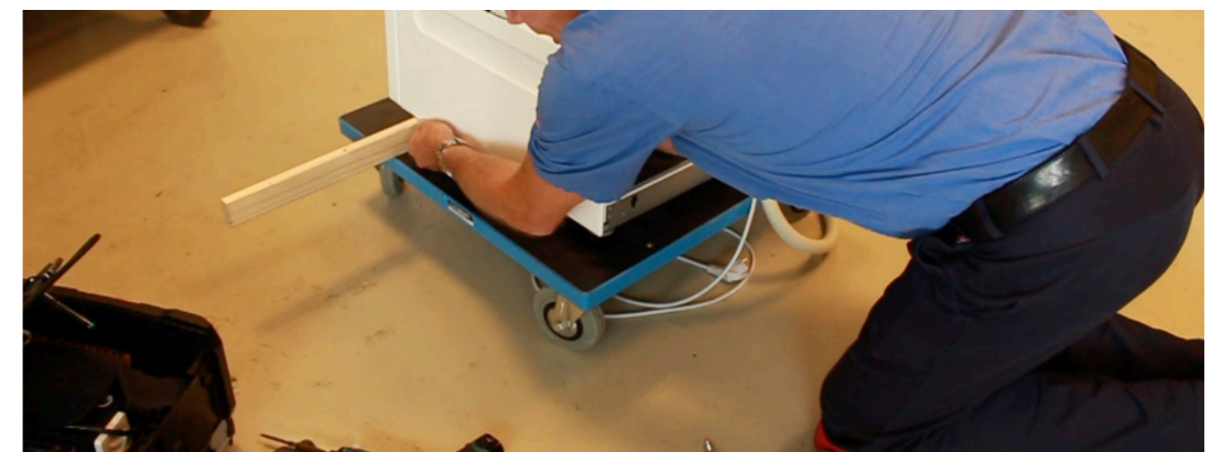
Image 17. Lack of visibility and extension of both arms needed to reach and release the component.
