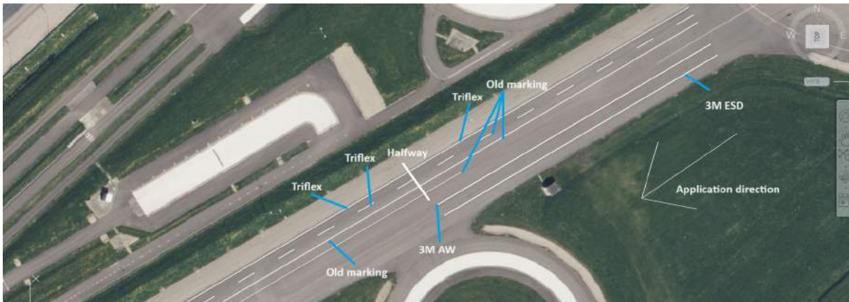
Figure 21: Placement of lane markings
