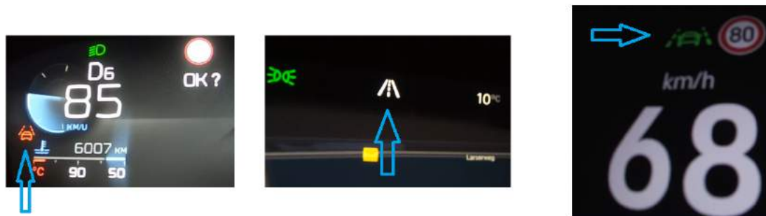
Figure 24: Left: Car A dashboard, Middle: Car B dashboard, Right: Car C dashboard. Blue arrow indicates the position of the LKA indicator symbol.
