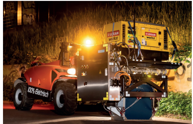
Figure 2 10kN Storm eVibe attached to electric Manitou MTE625.
