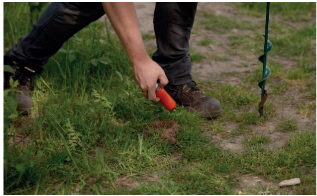
Figure 5 Stryde Node being deployed.
