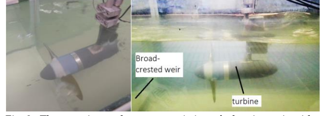
Fig. 3. The experimental set-up, consisting of a barrier weir with a two-bladed Tocado Power Turbine (scale 1:9, rotor diameter = 0.4 m) in a flume of the Environmental Fluid Mechanics Laboratory of Delft University of Technology.
