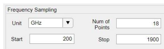
Figure 3.18: Frequency sampling section of the QO channel interface where the frequencies for which the QO channel model need to be simulated are specified.
