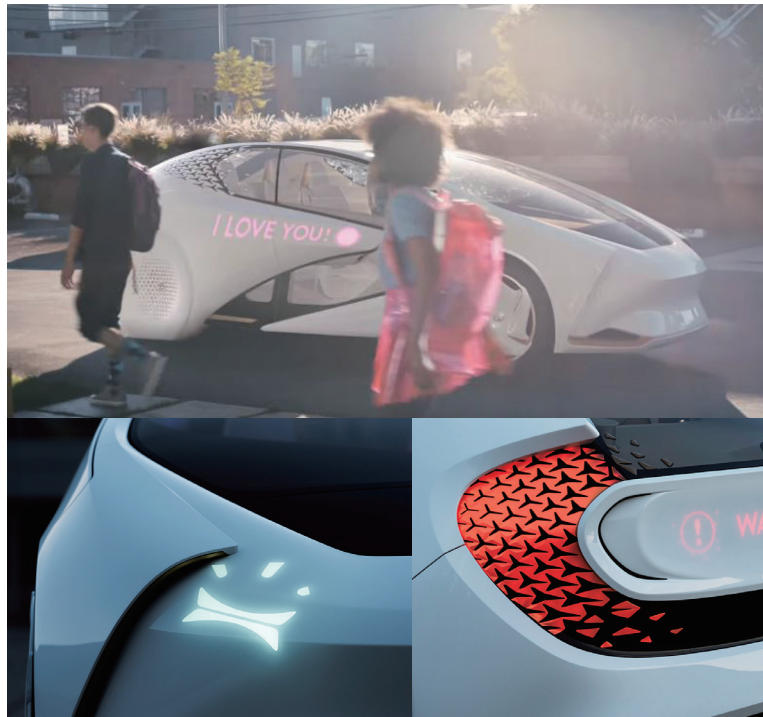
Figure 19 - V2P communication on Toyota concept car i
