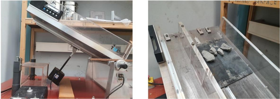
Figure 4.7: Inclined surface tester, side view (left) and top view (right)
