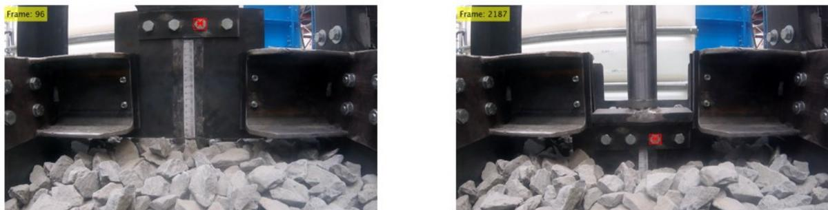
Figure 4.4: Video tracking tool applied for the penetration test, at the start (left), at the end (right)
