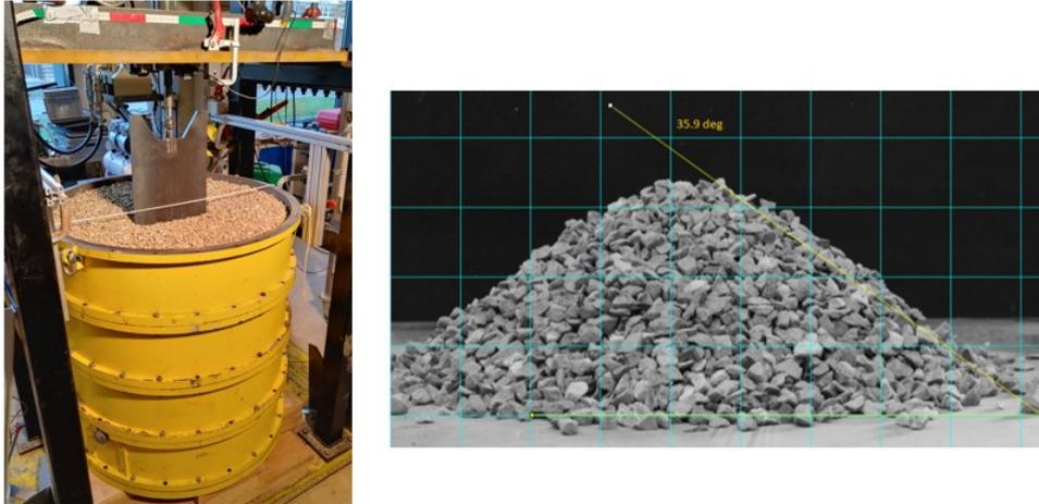
Figure 3.8: Laboratory experiments of a plate penetrating in granular material (left) and angle of repose (right)
