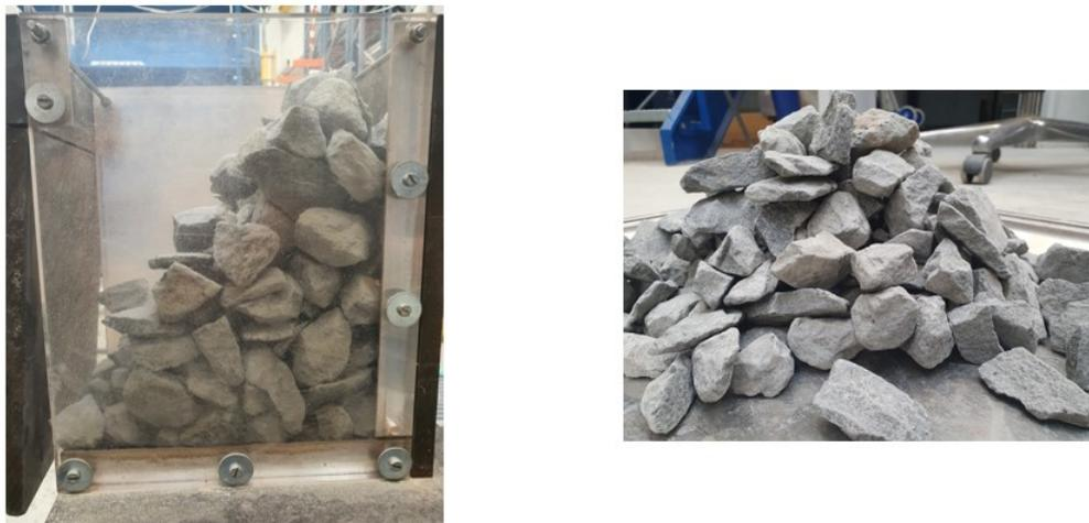
Figure 4.8: Angle of repose tests: shear box with opened door (left) and lifted cylinder pile of material (right)
