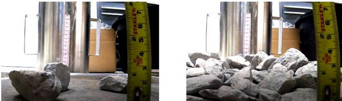
Figure 4.6: Drop test on a plate (left), on a pile of rocks (right)
