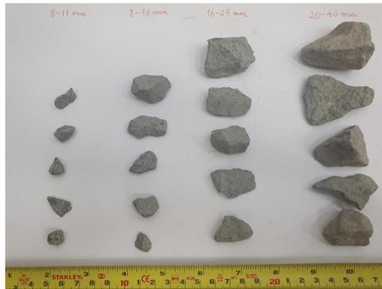
Figure 4.3: Representative samples of the basalt rock fragments
