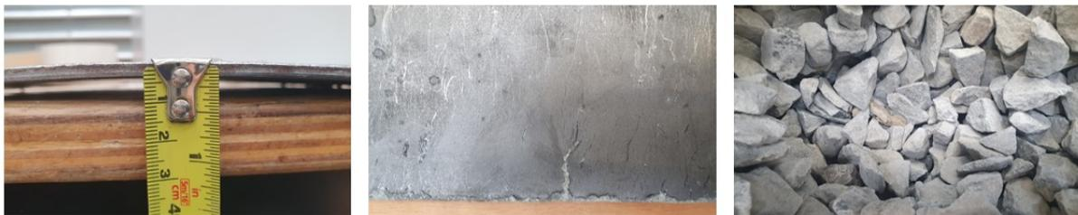
Figure 4.12: Buckled plate during the most extreme loading case (left), abrasion marks on the plate (middle), breakage of rocks (right)
