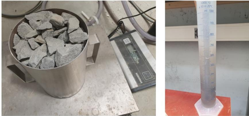
Figure 4.5: Bulk density container filled with rock material (left) and graduated water cylinder (right)
