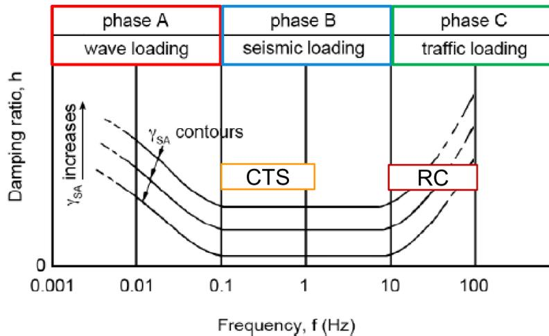
Figure 5: Small strain frequency dependence [29]
