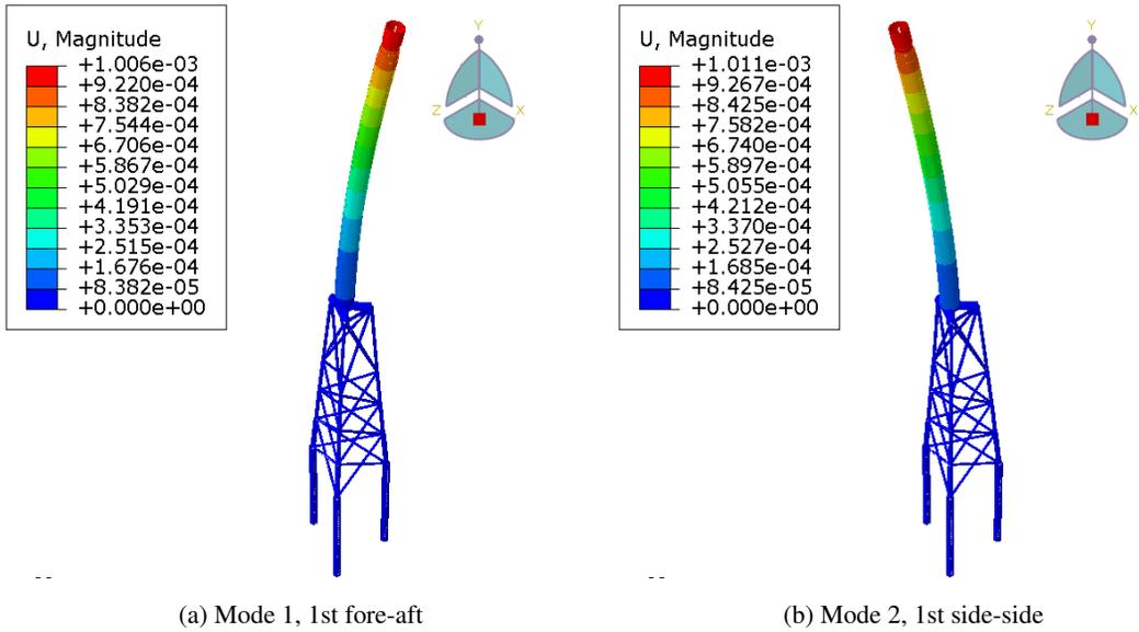
Figure 39: 1st set of bending modes
