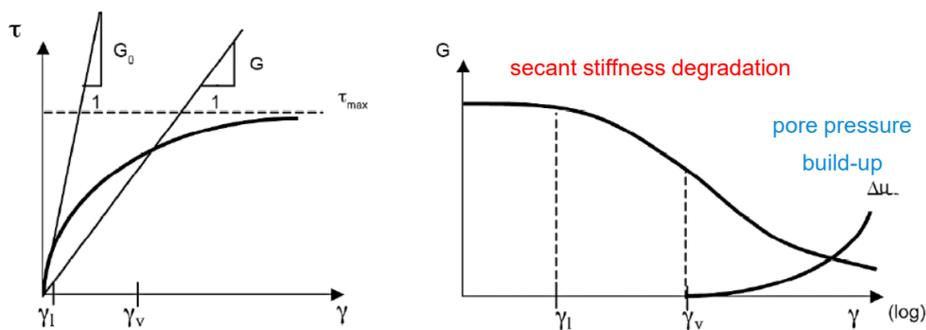
Figure 3: Soil strain characteristics [29]
