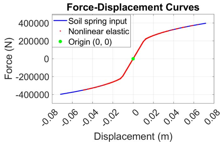
Figure 28: Input vs Nonlinear-elastic Force-displacement
