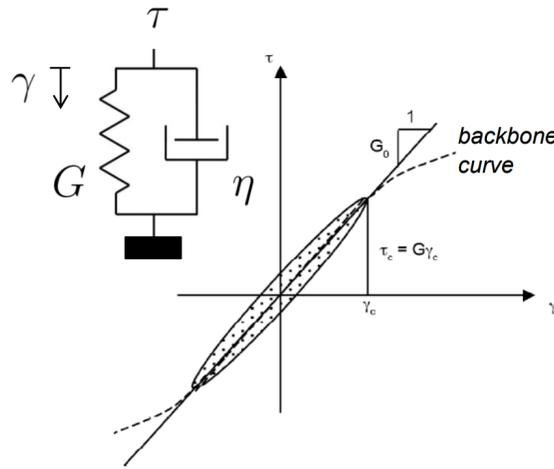
Figure 4: Small strain damping [29]
