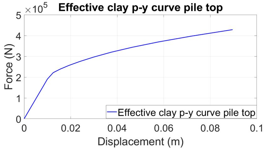
Figure 35: Effective clay p-y curve pile top till relevant displacement
