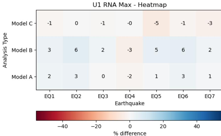
Figure 47: U1 RNA Max difference with respect to Model D
