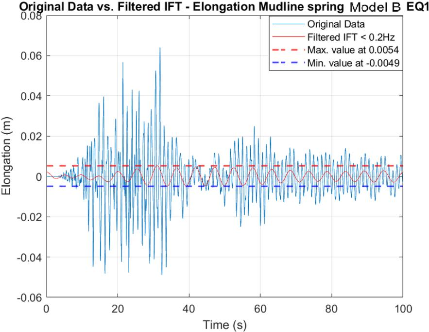
Figure 62: Elongation mudline spring total response & contribution  $< 0.2\text{Hz}$  - elastic model EQ1
