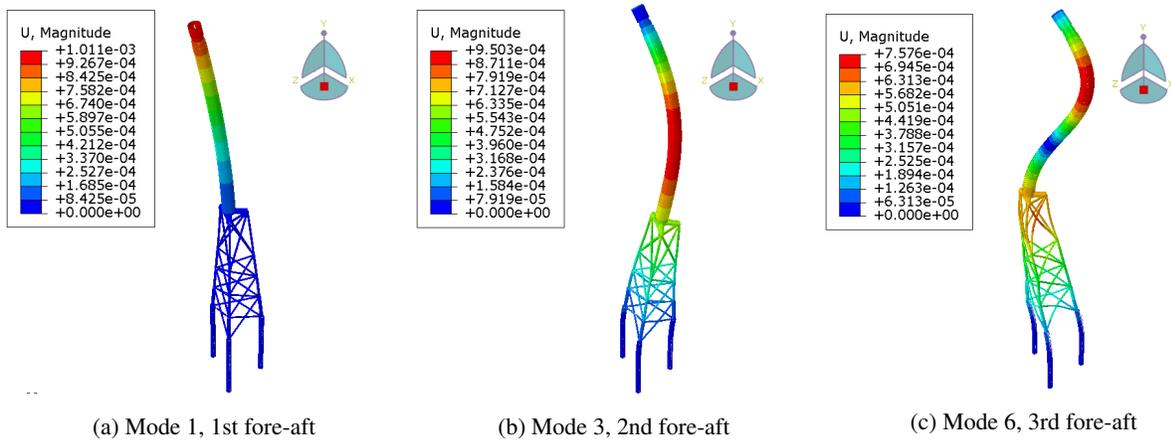
Figure 69: x direction tower bending modes
