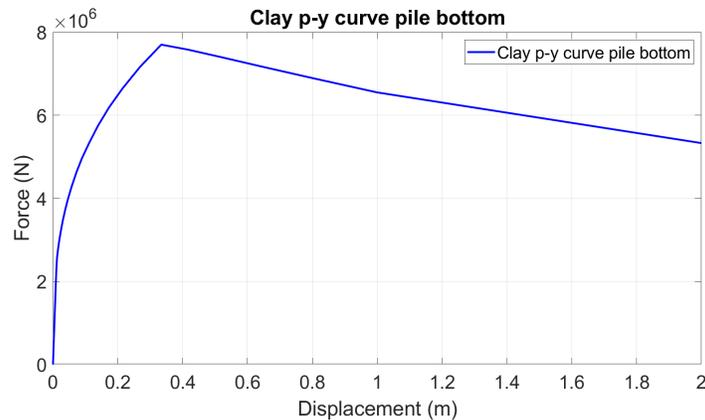
Figure 18: Clay p-y curve pile bottom
