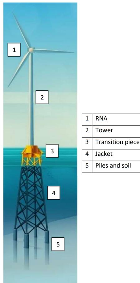
Figure 11: Parts of the structure [33]
