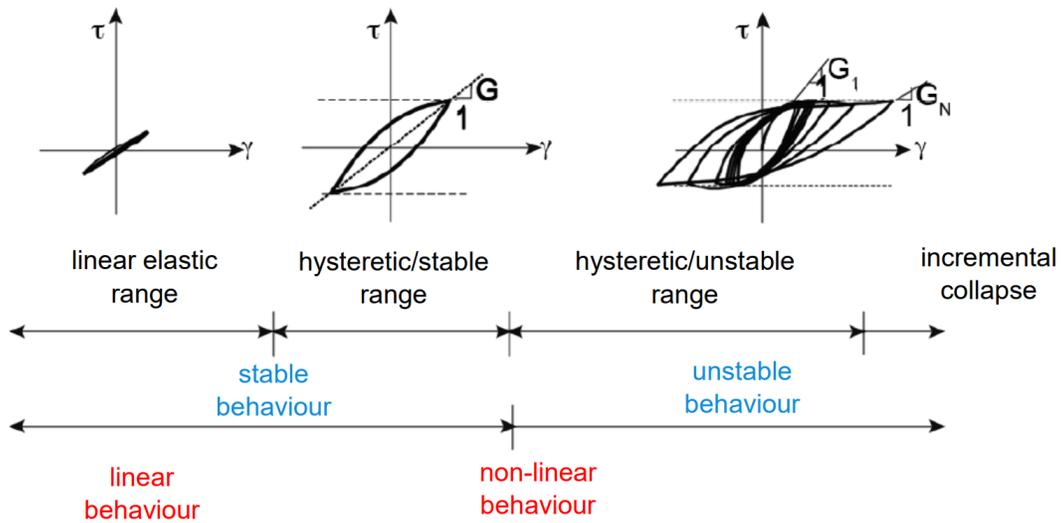
Figure 2: Soil strain characteristics [29]
