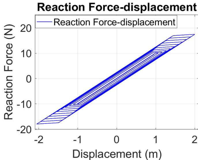
Figure 26: Force-displacement of plastic spring
