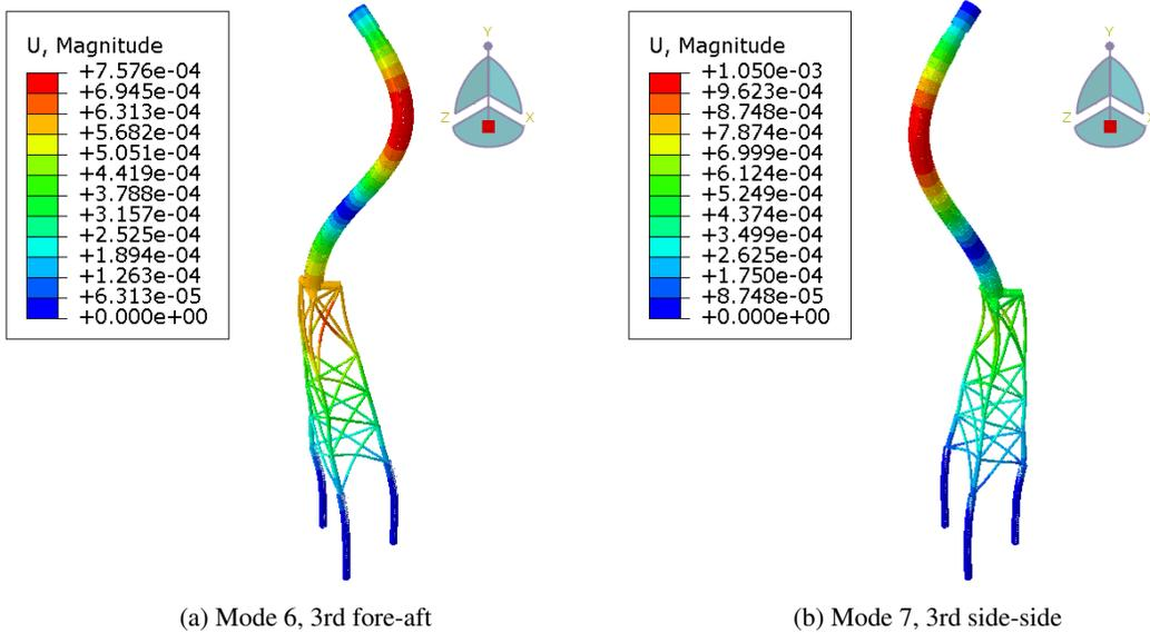
Figure 42: 3rd set of bending modes
