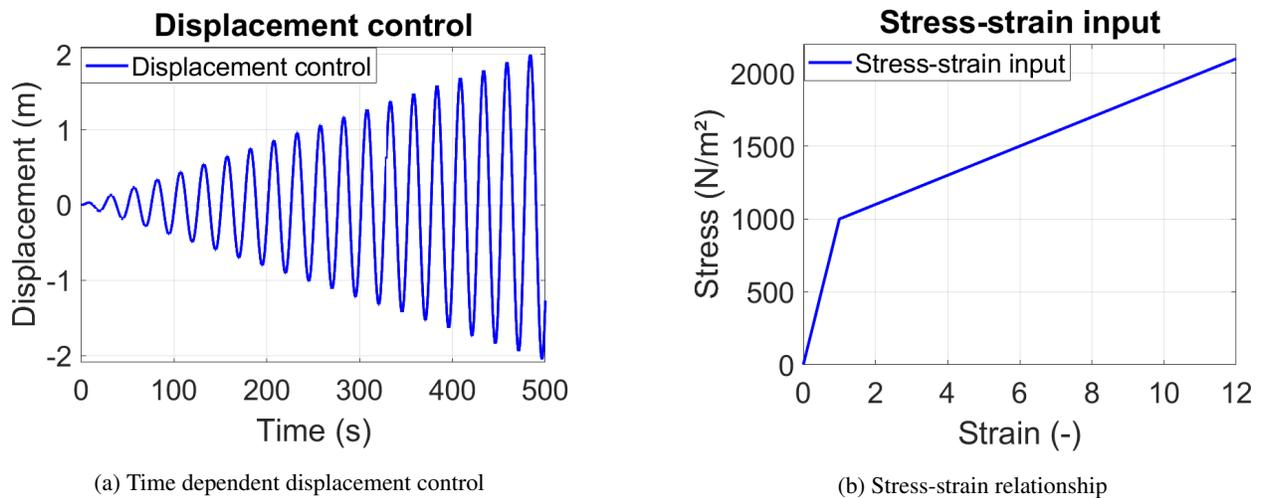
Figure 24: Loading and material input plastic spring
