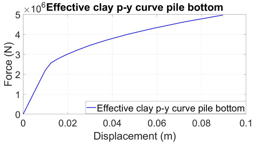
Figure 36: Effective clay p-y curve pile bottom till relevant displacement
