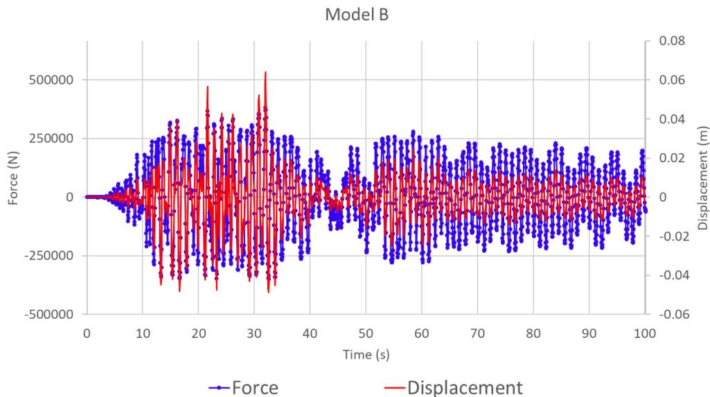
Figure 32: Model B Force (blue) & Displacement (red)
