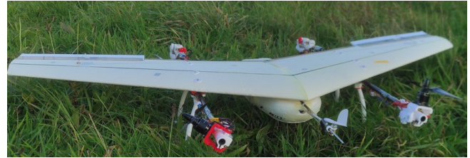
Figure 1: A picture of the dual-axis tilting rotor quad-plane developed at the TUDelft MAVLab.
