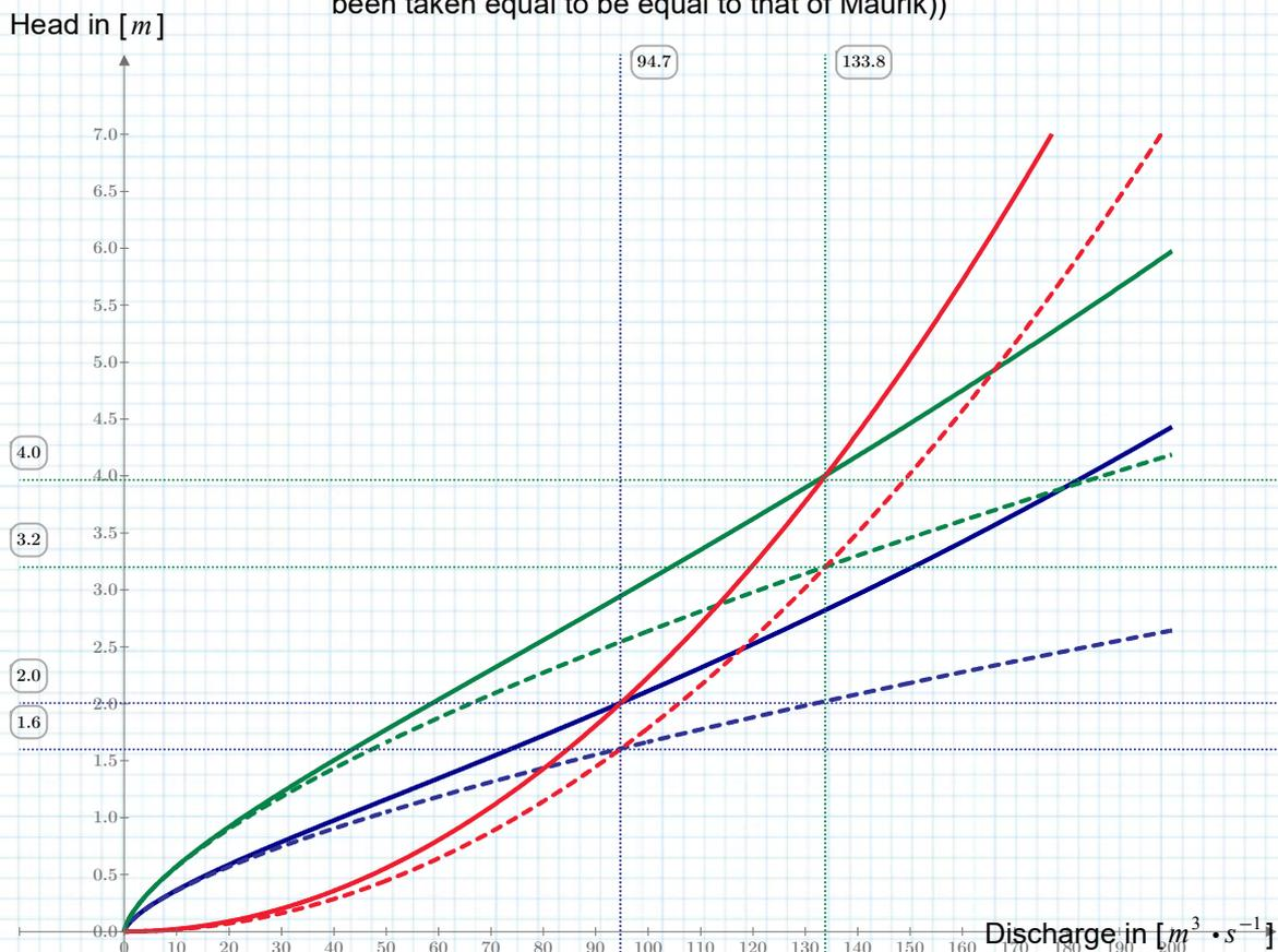
**Note:** By changing the specific speed, the system head differences  $H_{sum1}$  and  $H_{sum2}$  can be made to coincide for instance with the blue curve at the 2m.
