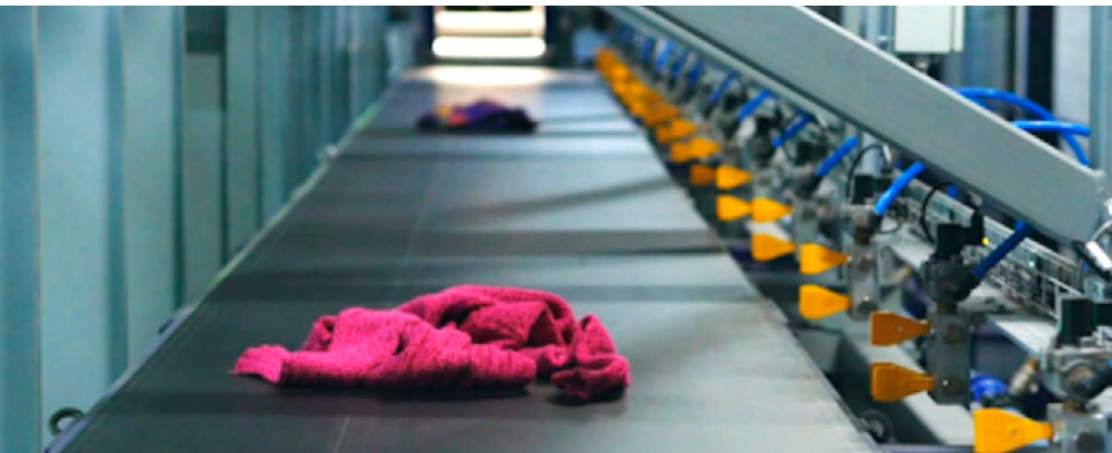
Image 3. The fiber sort machine of Textiles2Textiles sorts the garments based on color, structure and material (Wieland Textiles, n.d.).
