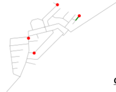
Figure 7.8: The optimal placement of four pressure sensors (at nodes N18, N20, N37 and N46) for detecting leaks of 15mm.
