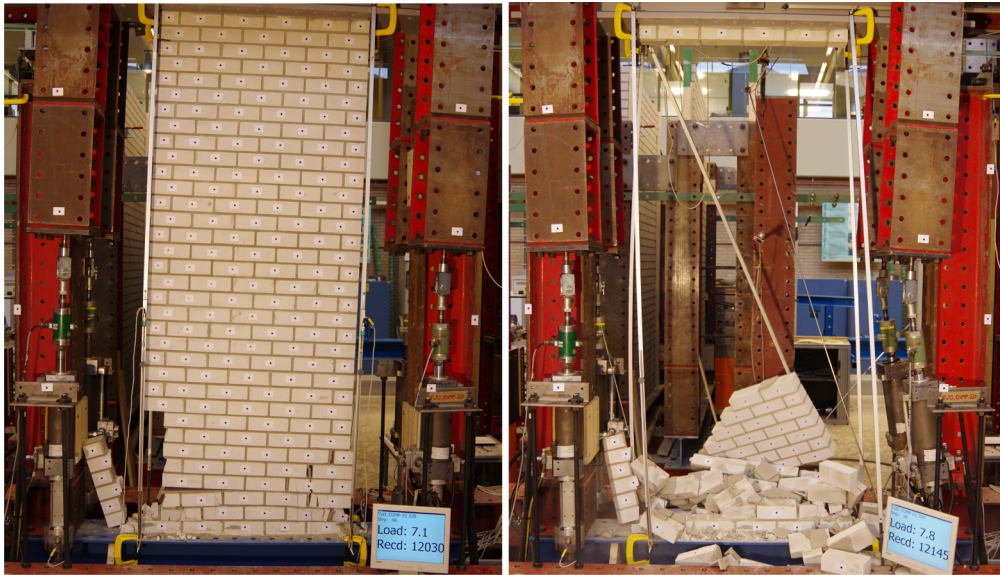
Fig. 5. Failure pattern of masonry wall in the TUDCOMP20 experiment before collapse (left) and after collapse (right) [29].
