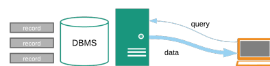
(b) Database approach (openDAP): Files are stored in database and only requested data are transferred
