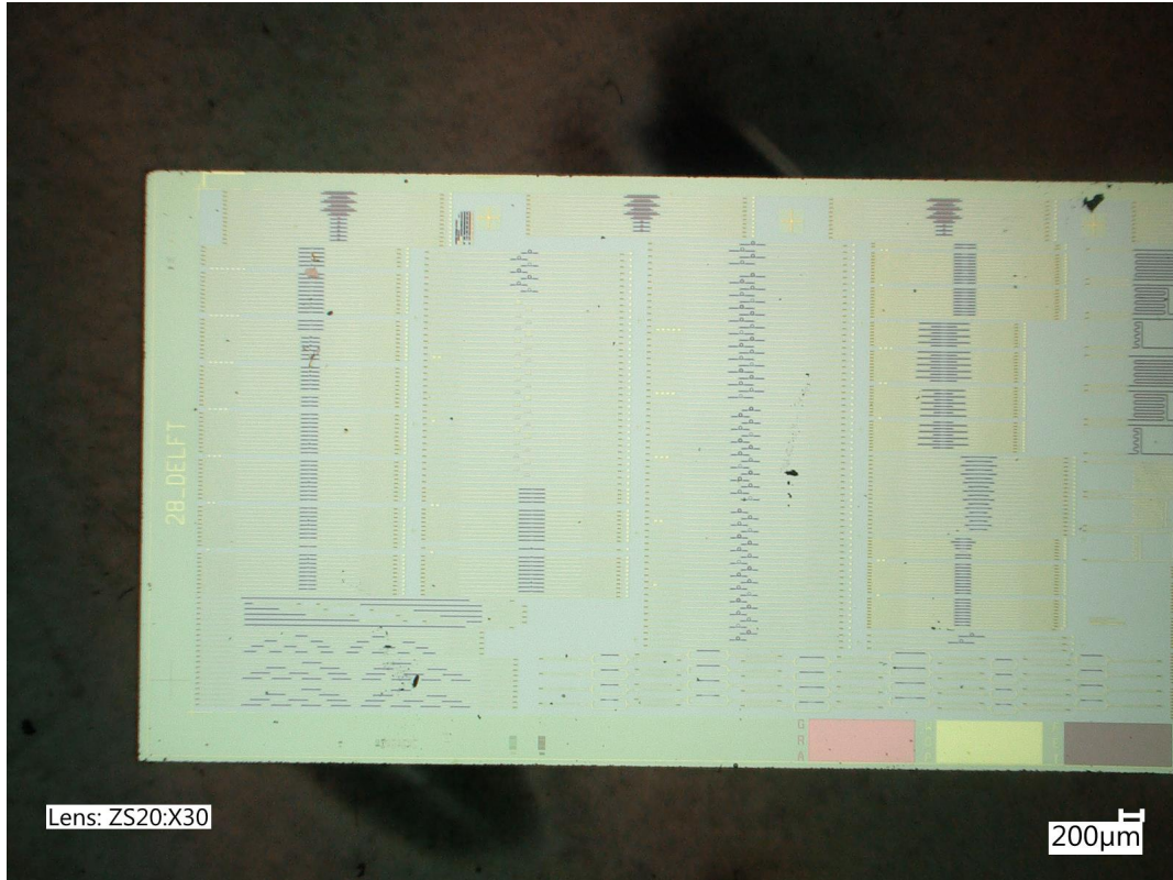
Figure 1: The silicon photonic chip used throughout this study. The left to center-right side of the silicon chip can be seen here. The circular and doughnut devices are in the first three central columns from the left. The left most column exclusively contains circular devices. The center column starts with doughnut shaped devices and ends with circular devices and the final column is exclusively for doughnut shaped devices. Other devices seen in the figure are, bus ring resonators on top with corresponding coupling gaps with a single ring resonator below the bus. A series of short straight waveguides are under the first column, these guides are used to measure internal transmission losses. Right of the short waveguides, are Mach-Zehnder interferometers. The fourth column contains a mixture of Bragg gratings and bus ring resonators with two doughnut membranes at the bottom.
