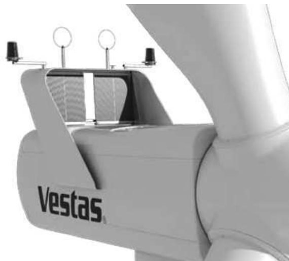
Figure 6.2: Vestas V80 [2], the radiator on top of the back of the nacelle obstructs the view of the radar.
