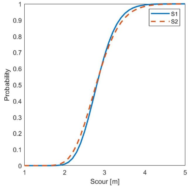
Figure 20. Fragility curve for the two foundations.
