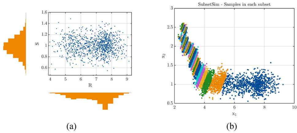
Figure 18. Process to obtain failure probability: (a) starting sampling (model uncertainties are not in the graph); and (b) subset simulation graphical process (where  $X_1$  is  $S$  and  $X_2$  is  $R$ ).
