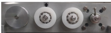
Fig. 2. Pulley system, from left to right: distance encoder, load cell, support pulley, stepper motor.
