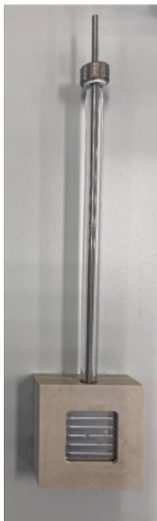
Figure 3.6: Electrodeposition holder
