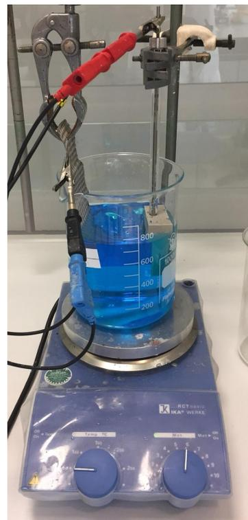
Figure 3.5: Electrodeposition setup for the catalyst synthesis
