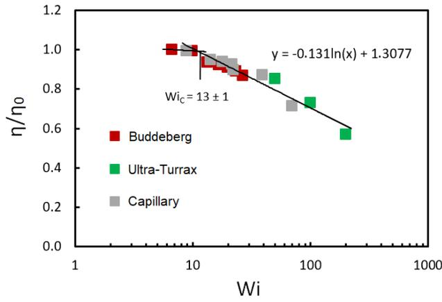
**Figure 3.** The normalized viscosity versus Weissenberg number. Red, green, and grey data points represent Buddeberg, Ultra-Turrax, and capillary respectively
