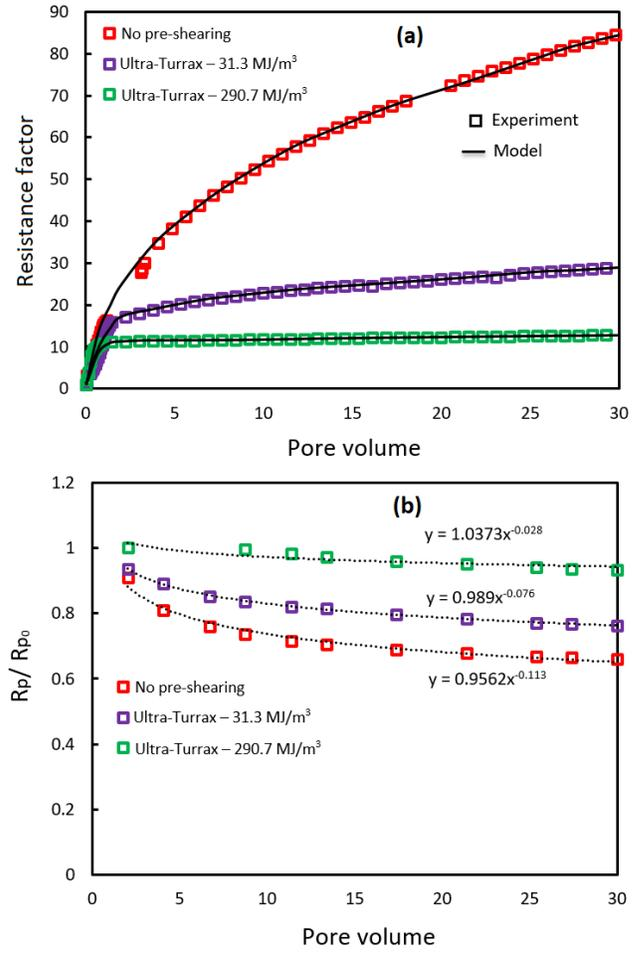
**Figure 6.** The sand-pack flow experimental and numerical modelling results. (a) Resistance factor ( $RF$ ) as a function of pore volume for the flow of un-sheared and Ultra-Turrax sheared polymer solutions at different energy input through the sand-pack and (b) reduction in the radius of pore throat ( $R_p$ ) as a function of pore volume
