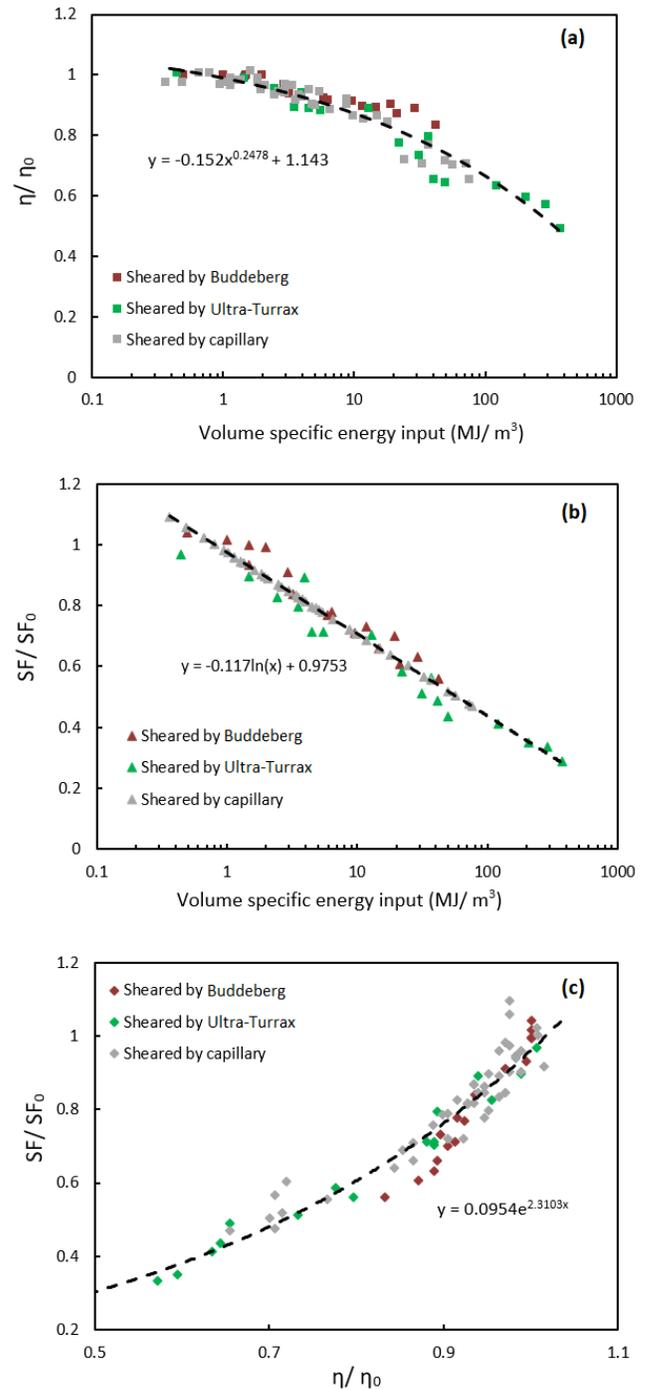
**Figure 4.** The change in viscosity and screen factor versus shearing intensity (based on the energy input) from the experimental series. (a) The normalized viscosity and (b) the normalized screen factor as a function of energy input and (c) the normalized screen factor as a function of the normalized viscosity. Red, green, and grey data points represent Buddeberg, Ultra-Turrax, and capillary respectively. The data presented here correspond to the data given in Figure 2
