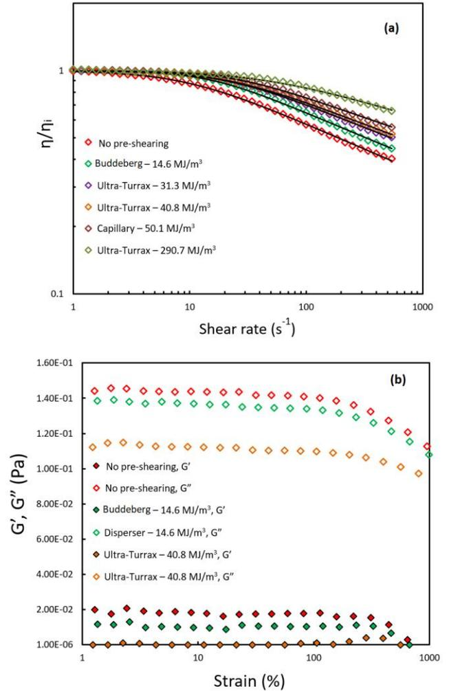
**Figure 5.** (a) The normalized steady-state shear viscosity of un- and pre-sheared polymer solutions. The solid line is acquired by fitting the experimental data into Carreau–Yasuda model. The fitting parameters are presented in Table S1 (see the supporting information). (b) The storage modulus ( $G'$ ) and loss modulus ( $G''$ ) as a function of strain at constant angular frequency  $\omega=6.28$  rad/s
