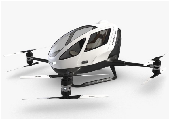
Figure 2.2: EHang-184 Coaxial Multi-rotor eVTOL [9]
