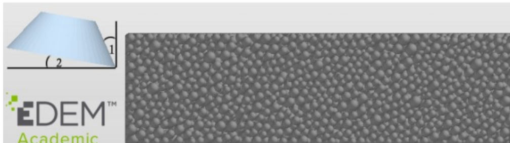
Figure 6 Clearance angle (2) and rake angle (1). (xz view, parallel to positive y axis)
