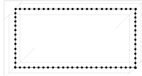
Figure 11.8: Discretisation of the cross section of the wingbox
