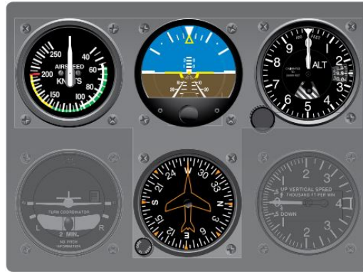
Figure 16.7: T-configuration of analog flight instruments
