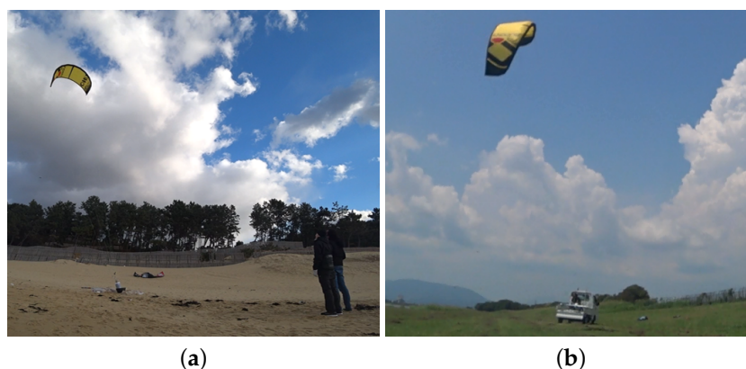
Figure 3. Flight tests with (a) stationary kite control unit (KCU) anchored at the ground and (b) towed KCU flying on a short tether.
