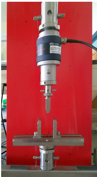
Figure 3.3: The Instron three-point bending test device
