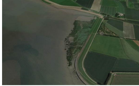
(b) Hellegat, salt marsh, Western Scheldt. Marsh elevation 3.0 m+NAP, width 200 m, slope 1:40. Dike height 9.5 m+NAP, slope 1:4. Design conditions: h = 6.0 m+NAP, H_{m0} = 1.9 m, T_{m-1,0} = 5 s.
