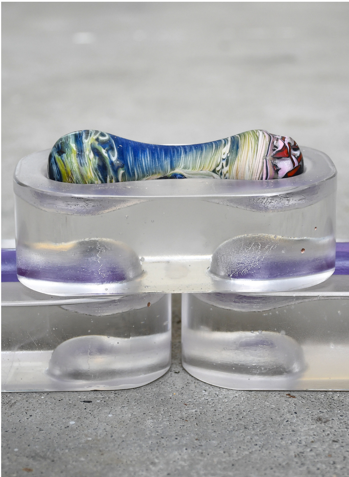
Re3 Glass: Research by Faidra Oikonomopoulou and Telesilla Bristogianni at TU Delft into a Reduce, Reuse and Recycle strategy for a dry assembly building system out of waste glass.
